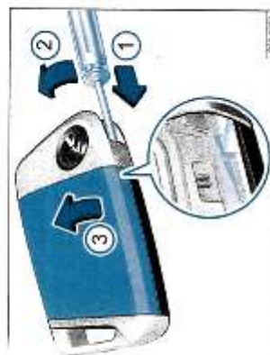
Fig. 55 Remote control vehicle key: Opening the battery compartment cover.
