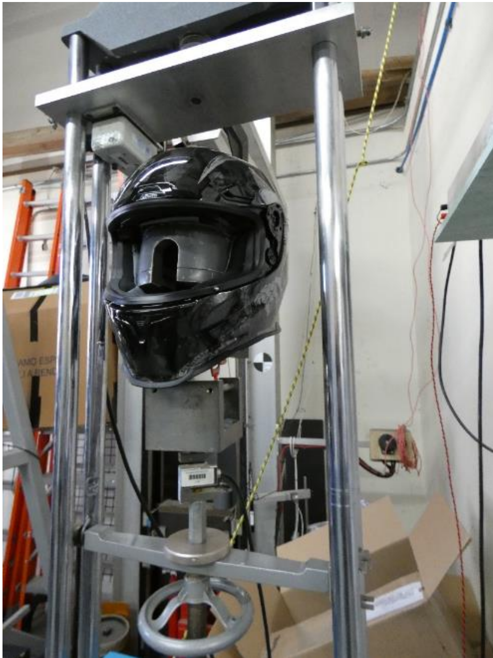
Pre-Test Photograph of Helmet Retention Test
