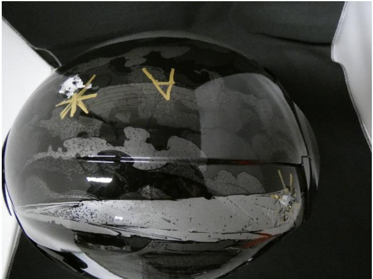
Helmet penetration test locations
