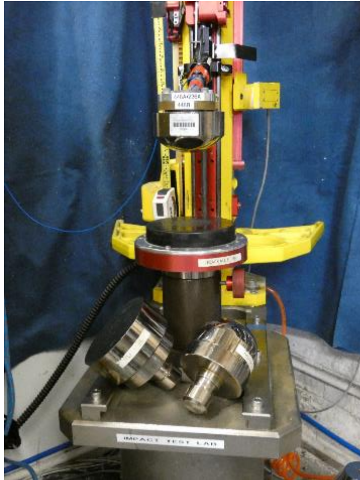
Impact attenuation test apparatus with flat, hemi and MEP anvils
