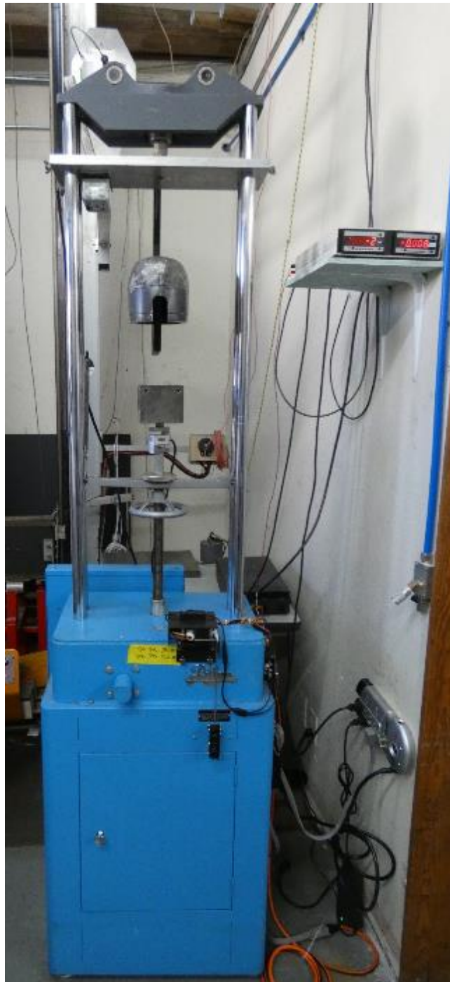
Retention system test apparatus with load cell and string potentiometer
