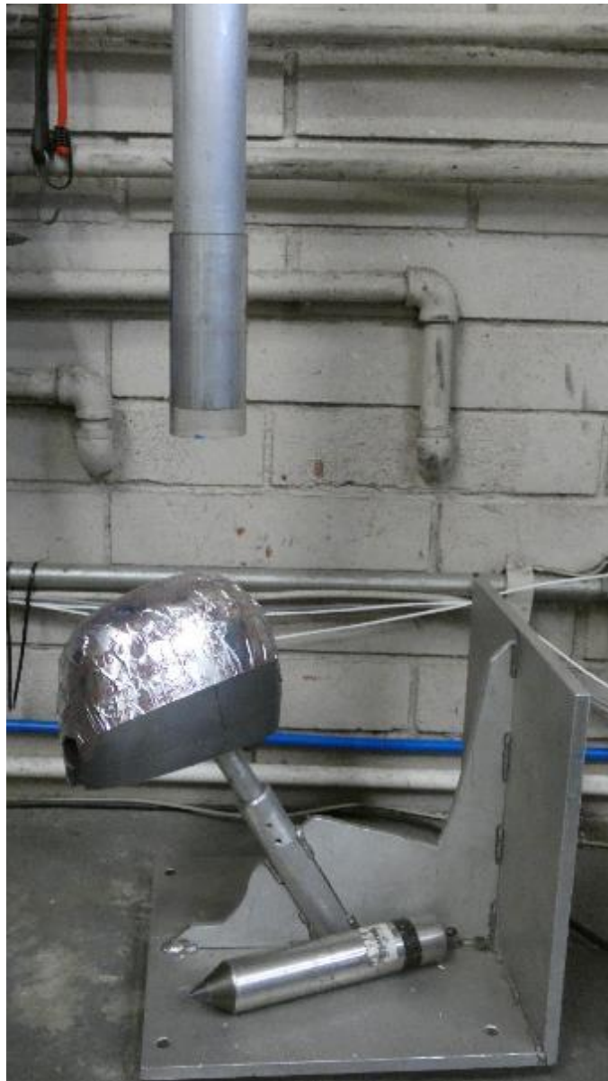
Penetration test apparatus with headform, penetration striker and adjustable base
