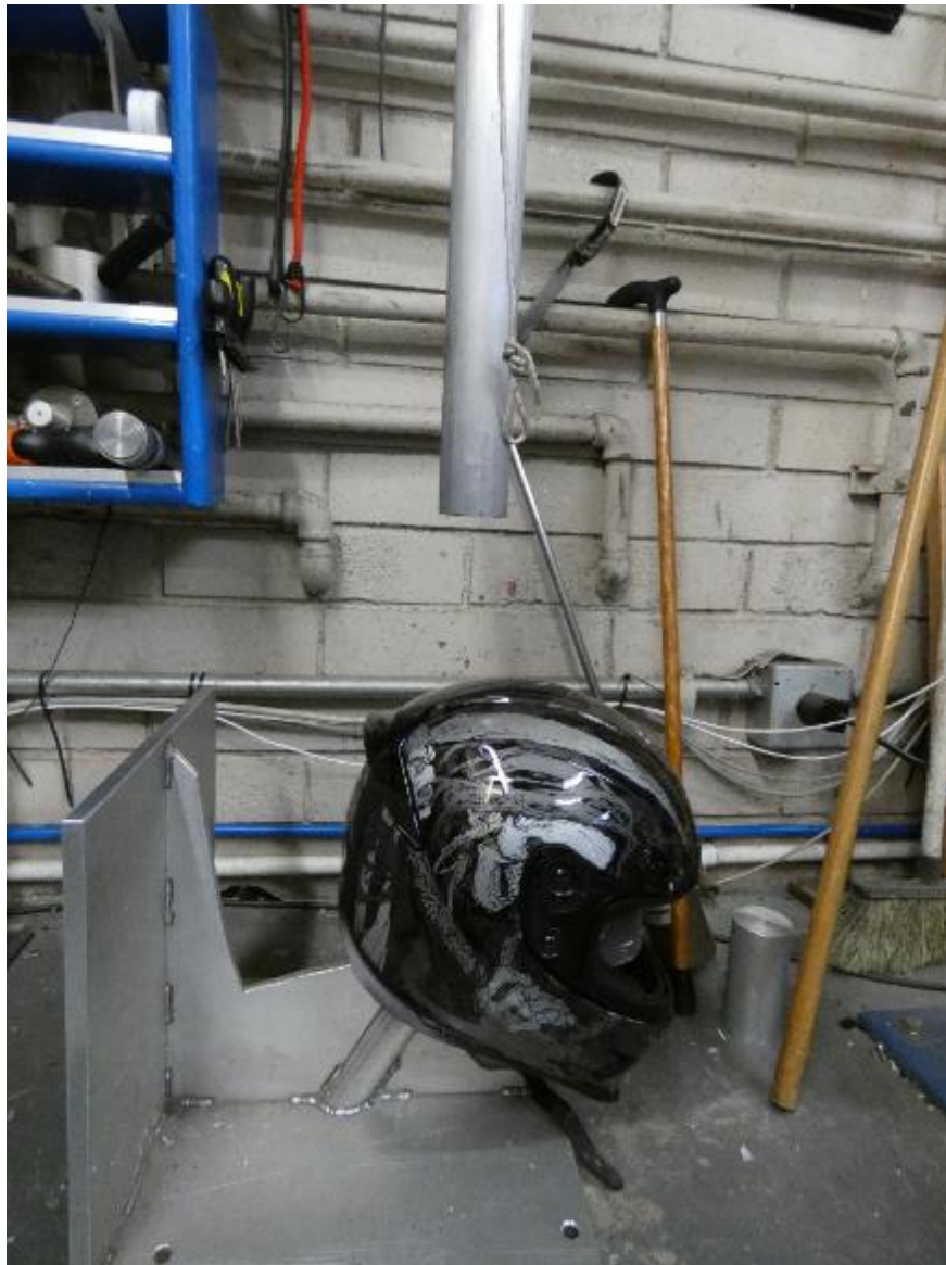
Pre-Test Photograph of Helmet Penetration Test
