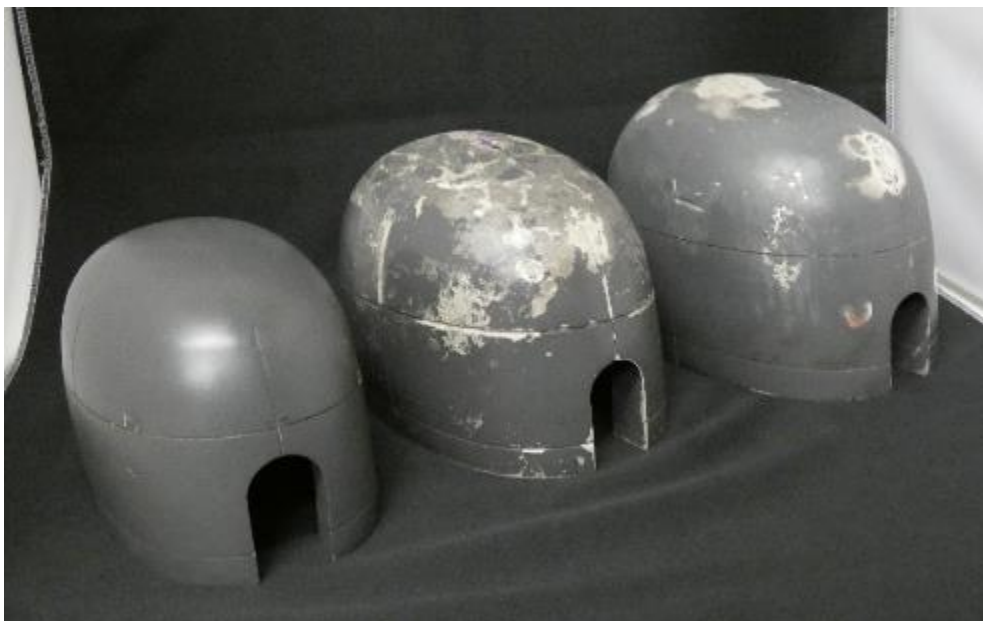
Impact test headforms (Small, Medium, Large)
