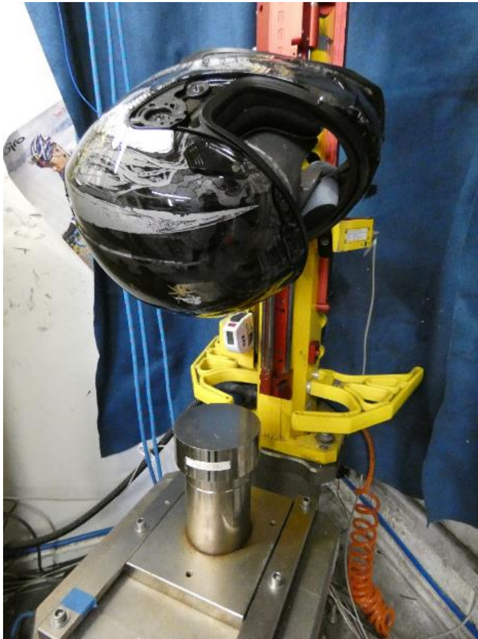
Pre-Test Photograph of Helmet on Monorail Test Rig
