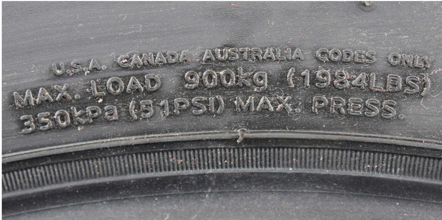
FIGURE 5.8 TIRE SHOWING MAX LOAD RATING AND MAX COLD INFLATION PRESSURE
