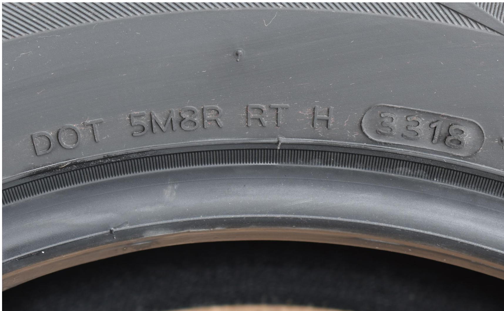
FIGURE 5.7 TIRE SHOWING DOT NUMBER
