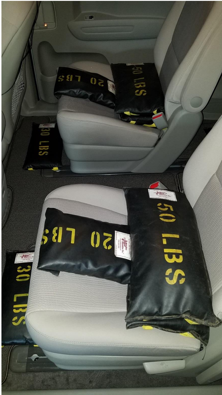
FIGURE 5.11 MID SEATS BALLASTED FOR UVW+VCW GAWR LOAD
