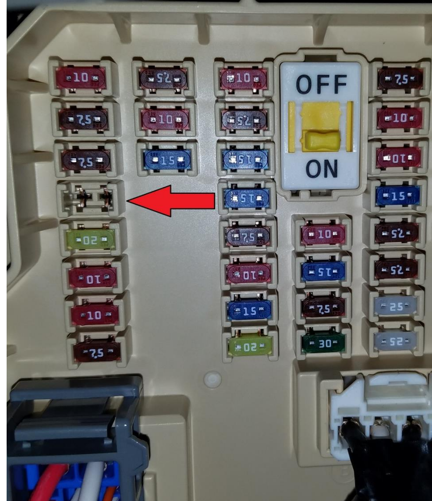
FIGURE 5.16 MALFUNCTION 2 – TPMS FUSE REMOVAL
