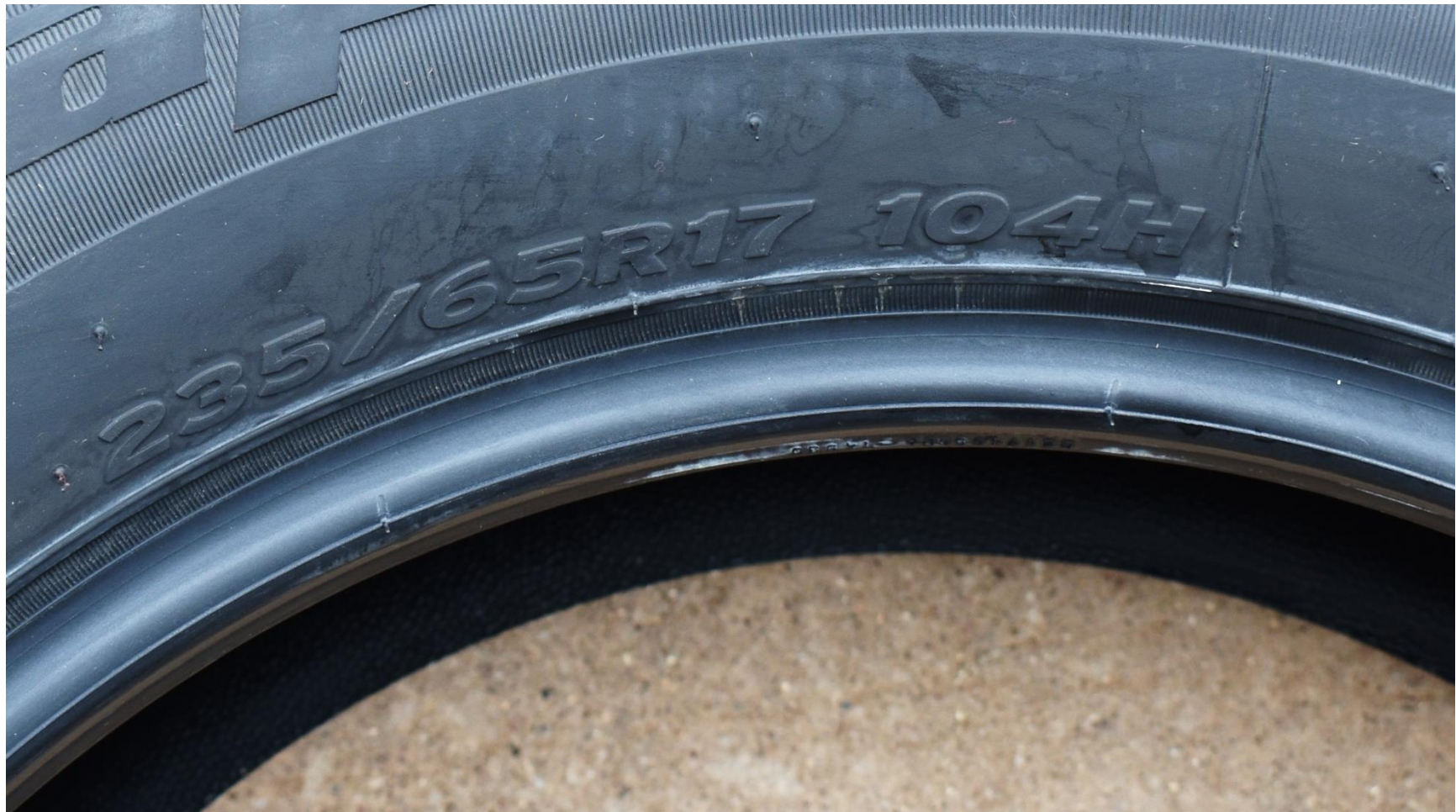
FIGURE 5.6 TIRE SHOWING SIZE AND LOAD INDEX /SPEED RATING
