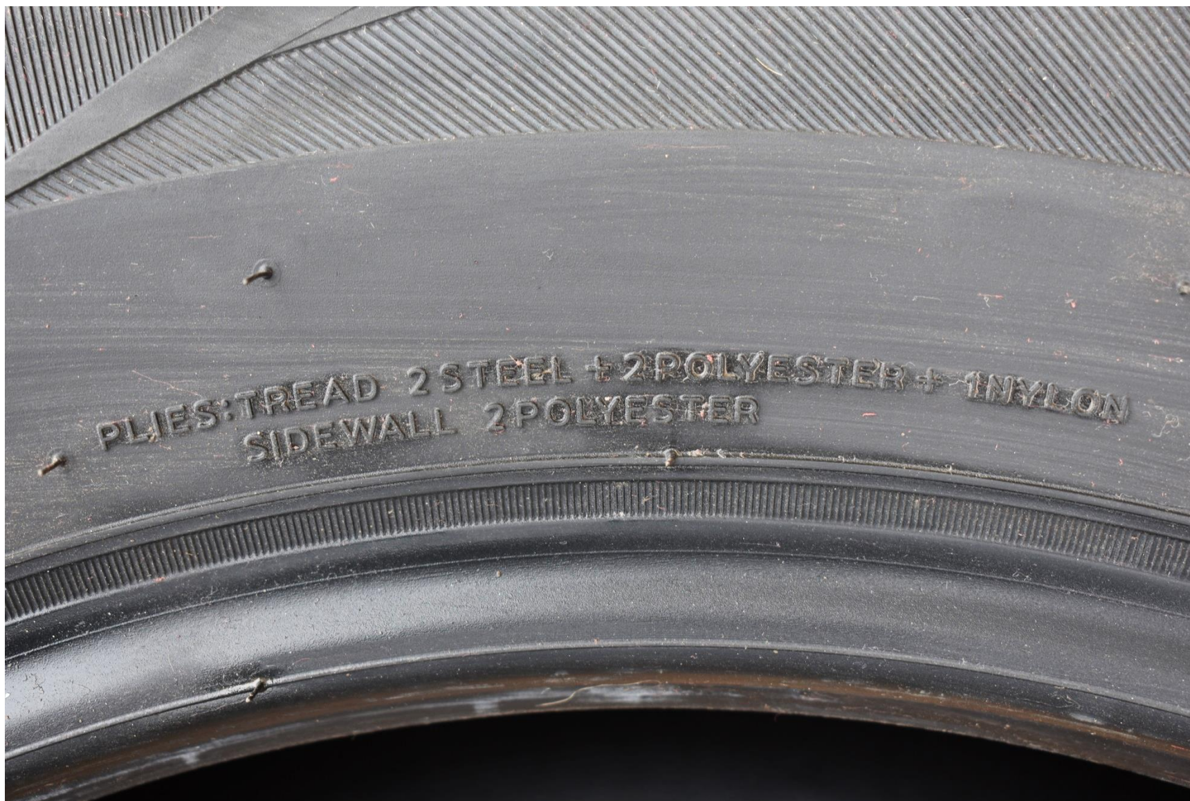
FIGURE 5.9 TIRE SHOWING SIDEWALL / TREAD CONSTRUCTION
