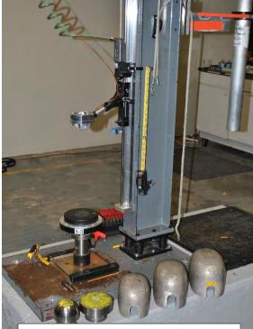
Impact attenuation test apparatus with three headforms (S, M, L), flat, hemi and MEP anvils
