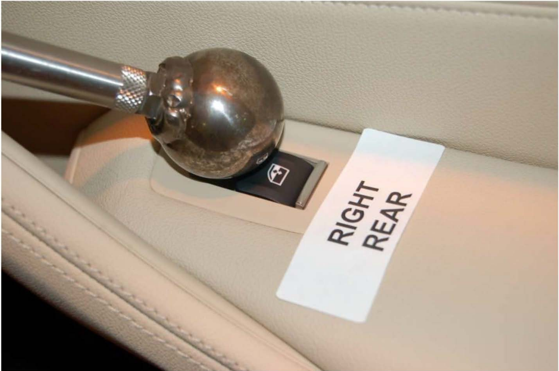
FIGURE 5.16 SPHERE TEST ON RIGHT REAR WINDOW SWITCH
