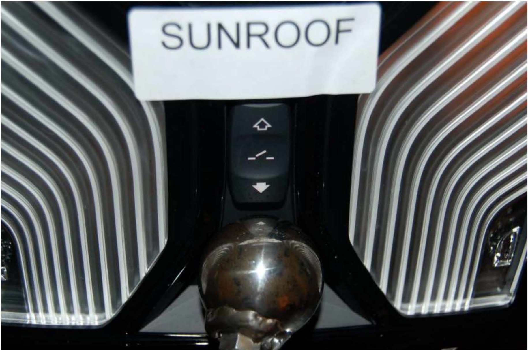
FIGURE 5.17 SPHERE TEST ON SUNROOF CONTROL SWITCH
