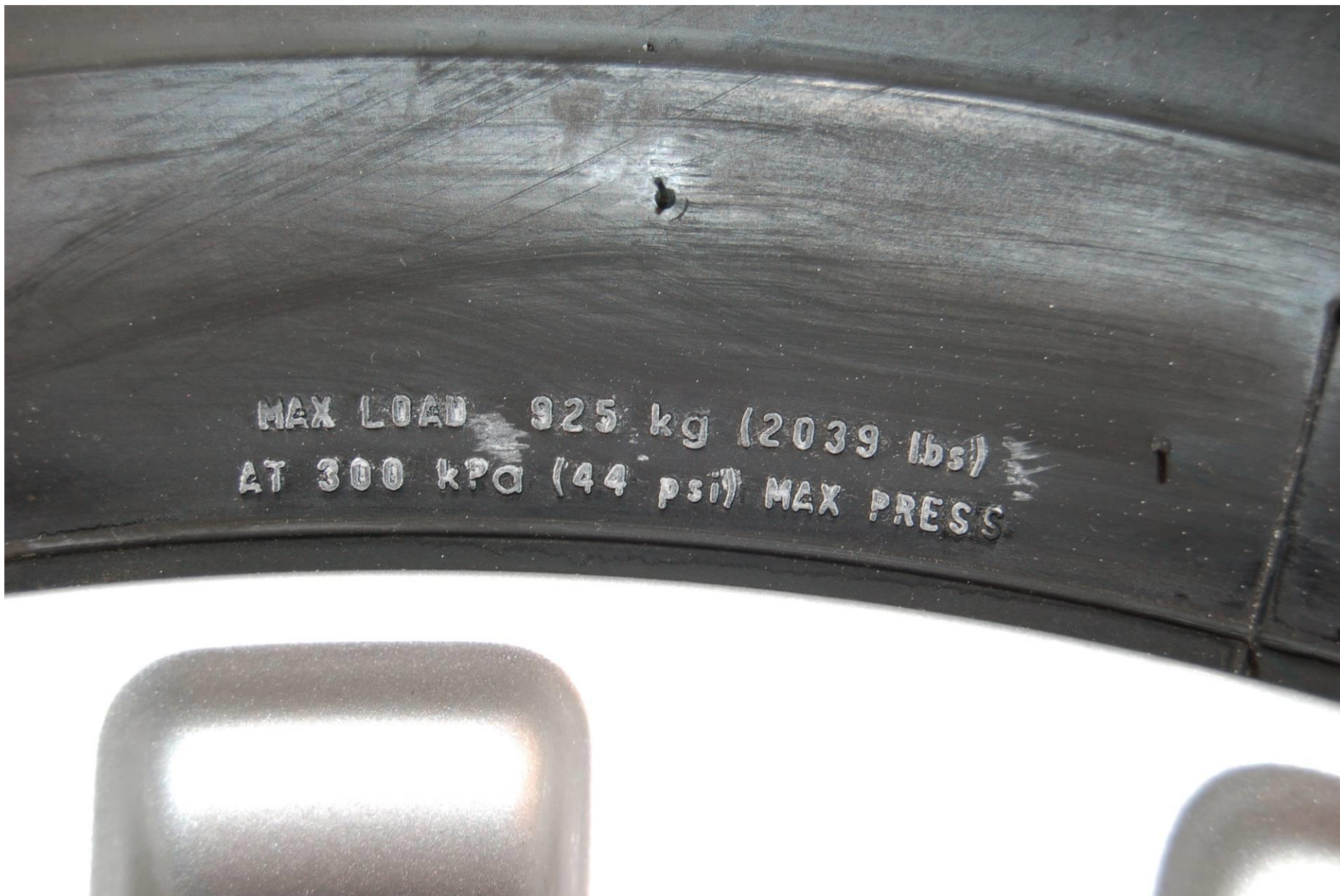
FIGURE 5.7 TIRE SHOWING PRESSURE AND LOAD RATING
