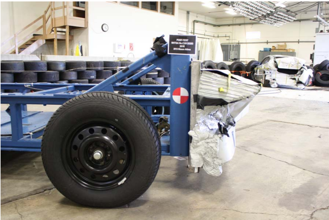
Figure A-24: Post-Test MDB Right Side View
