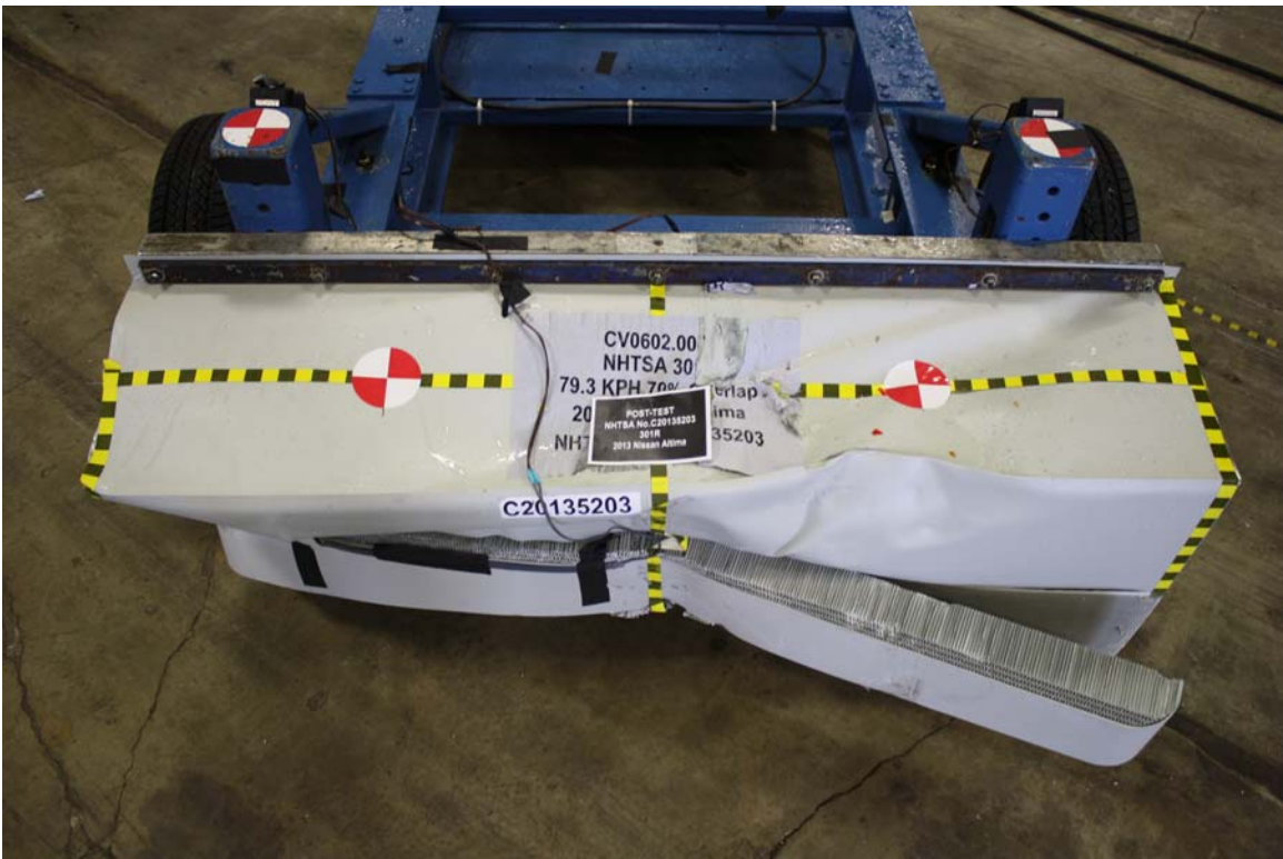
Figure A-26: Post-Test MDB Top View
