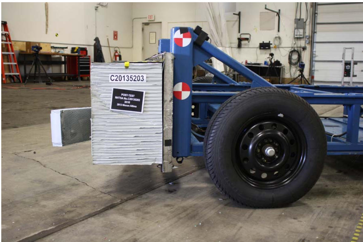
Figure A-22: Post-Test MDB Left Side View
