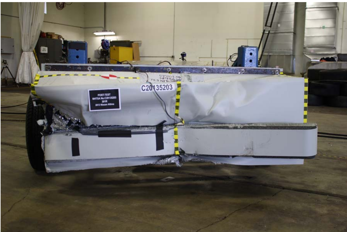
Figure A-20: Post-Test MDB Front View
