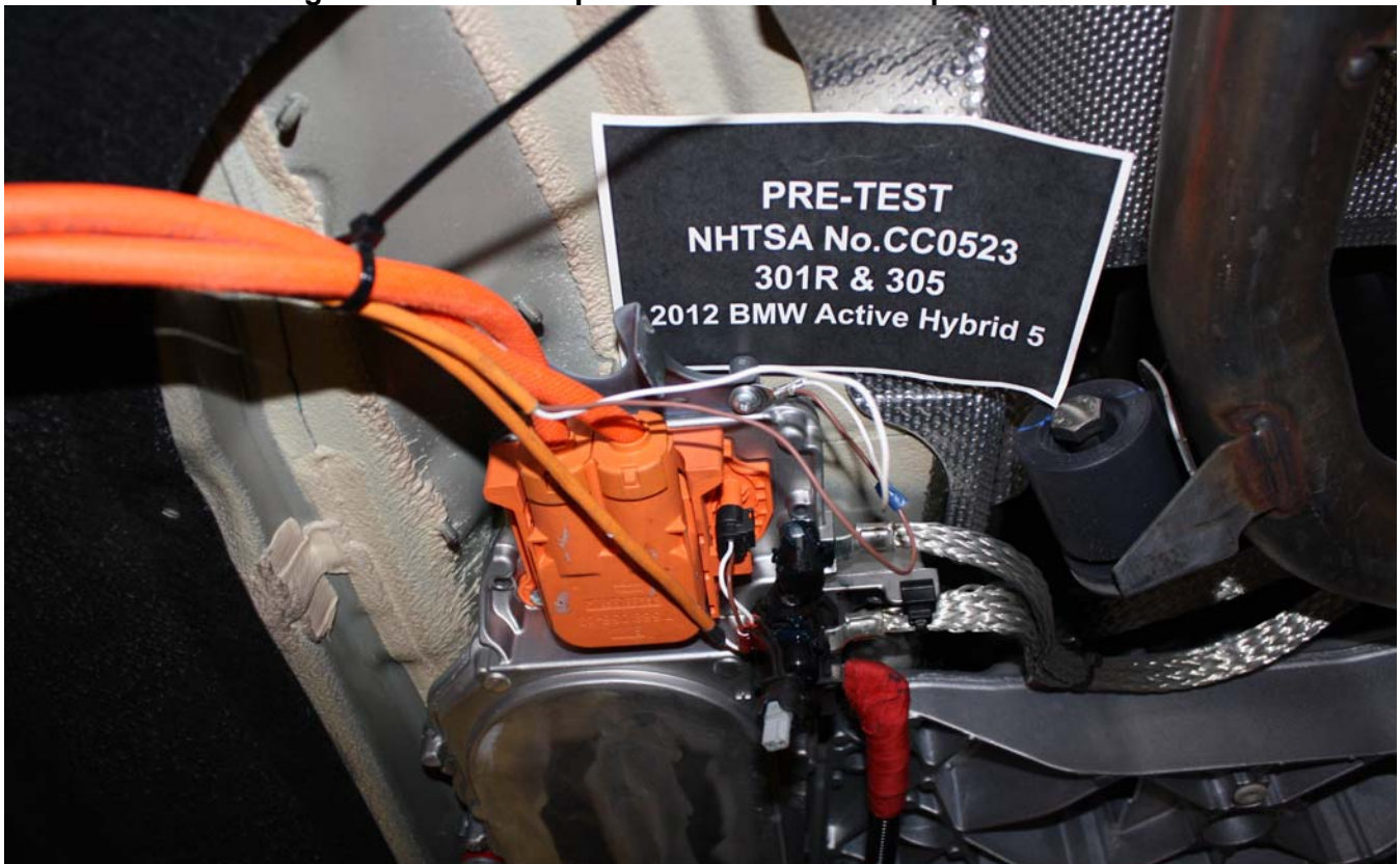
Figure A-58: Pre-Impact View of High Voltage Interconnect(s)
