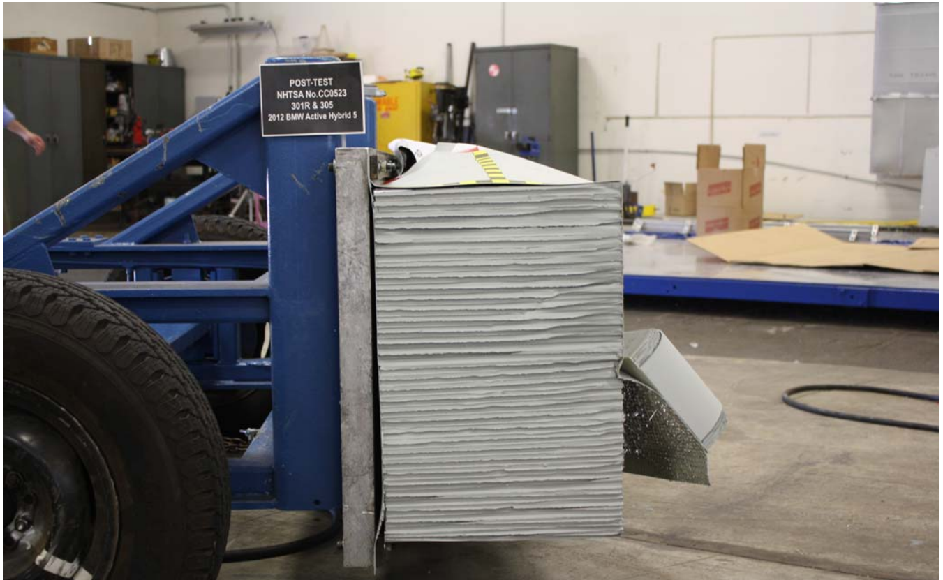
Figure A-26: Post-Test MDB Right Side View
