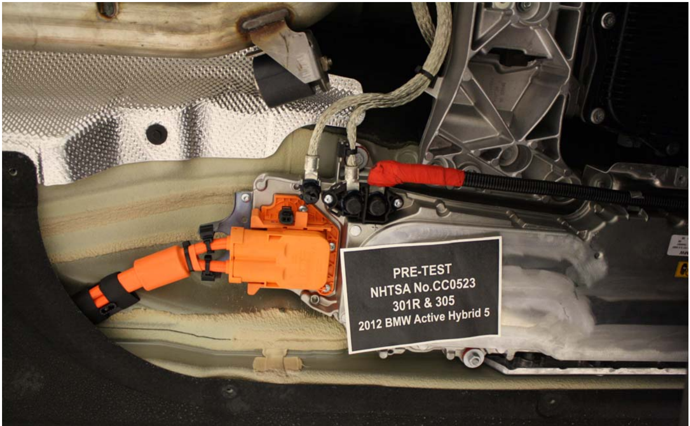
Figure A-63: Pre-Impact Close-Up View of High Voltage Leads Attached
