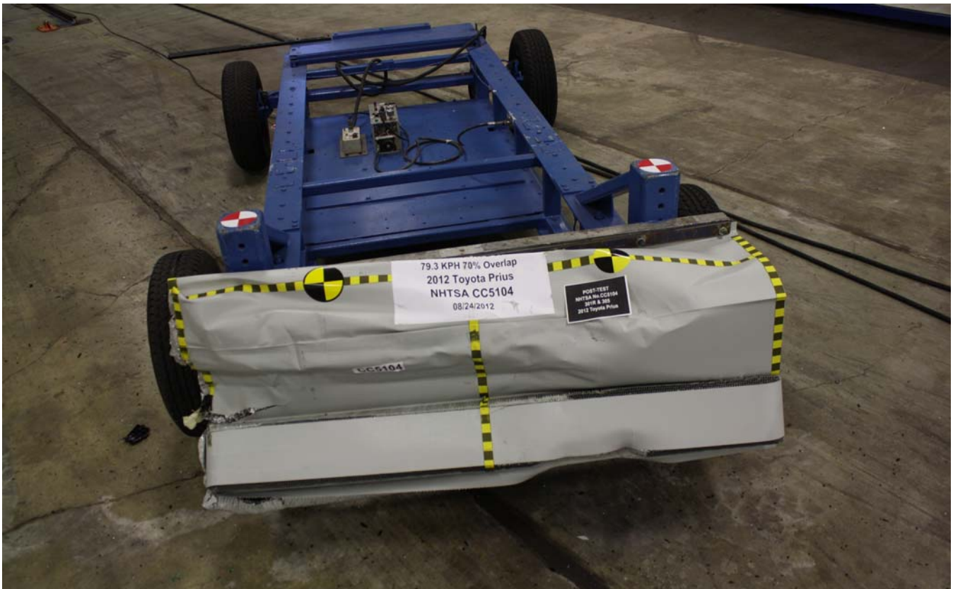
Figure A-28: Post-Test MDB Top View
