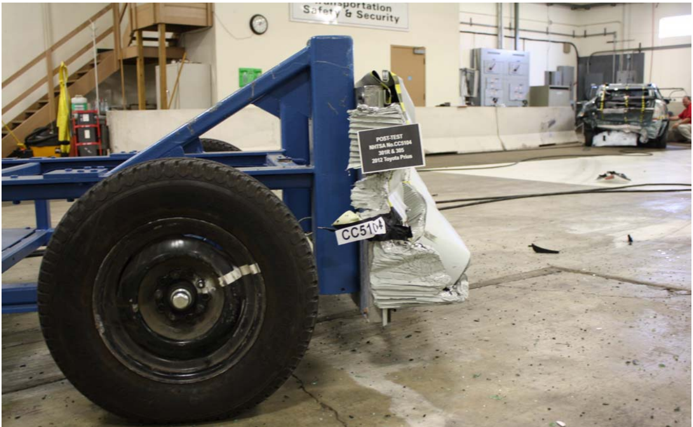
Figure A-26: Post-Test MDB Right Side View
