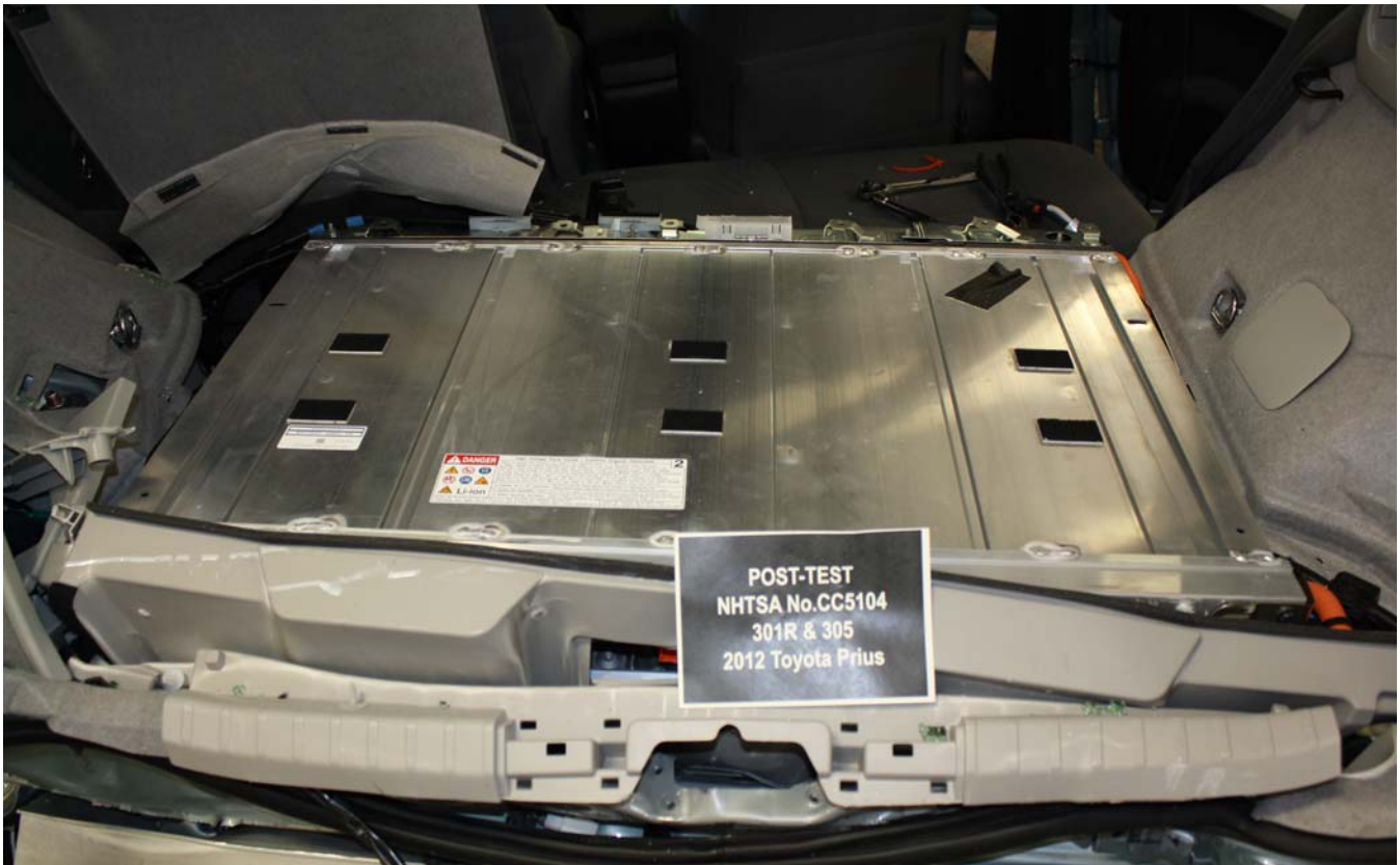
Figure A-51: Post-Impact Rear View of Propulsion Battery (if any part of it is visible)
