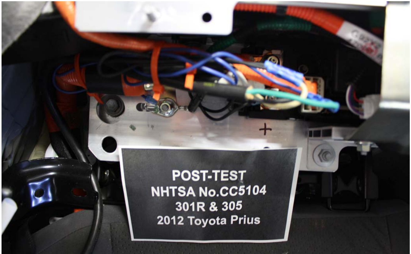
Figure A-65: Post-Impact View of Installed Test Interface Port
