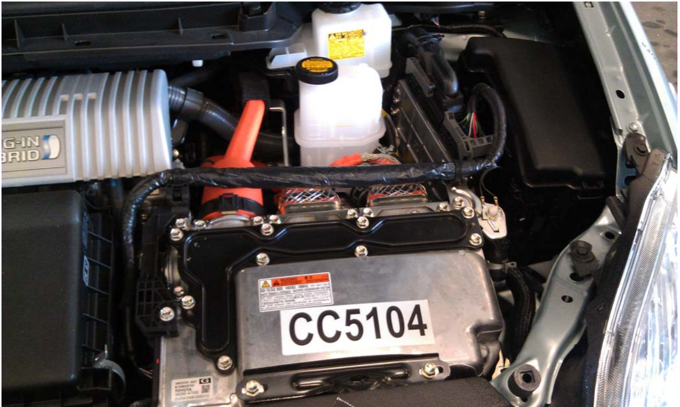
Figure A-57: Post-Impact View of Electric Propulsion Drive
