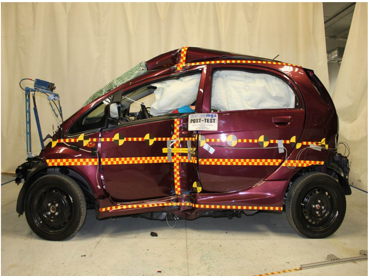
Post-Test Impacted Side View of Test Vehicle
