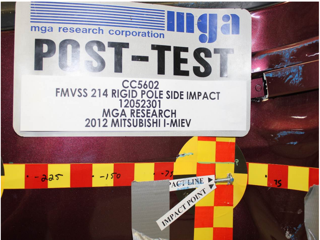
Post-Test Close-up View of Impact Point Target
