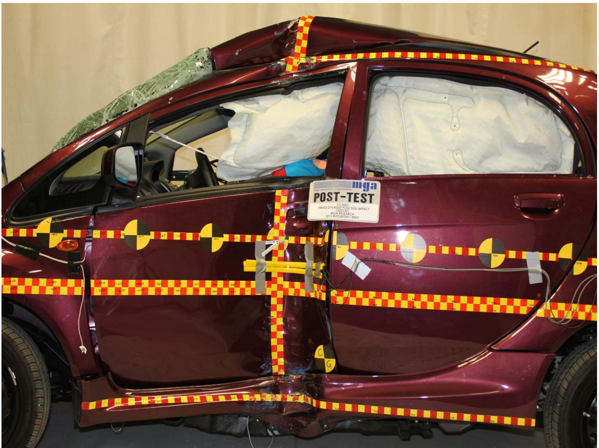
Post-Test Impact Zone Close-up View
