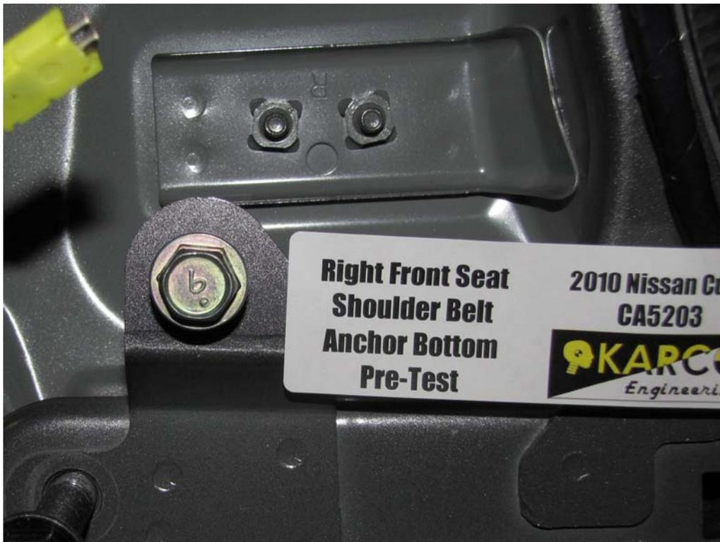
FIGURE 97. Shoulder Belt Anchor, P2, Pre-Test
