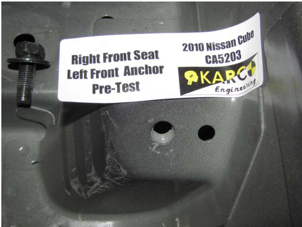
FIGURE 79. Floor Pan Anchor, P2, Pre-Test
