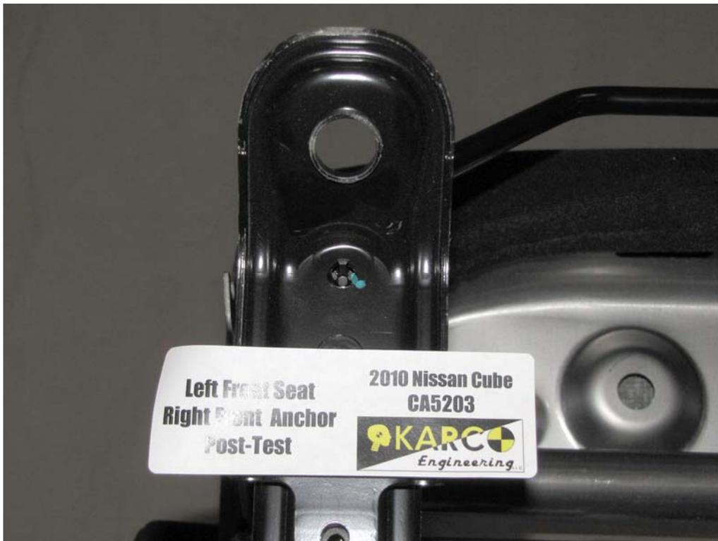
FIGURE 58. Seat Anchor, P1, Post-Test
