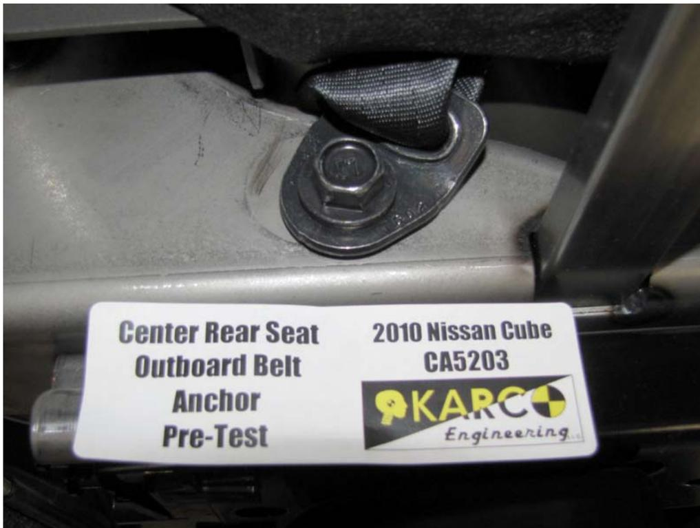
FIGURE 143. Belt Anchor, P6, Pre-Test
