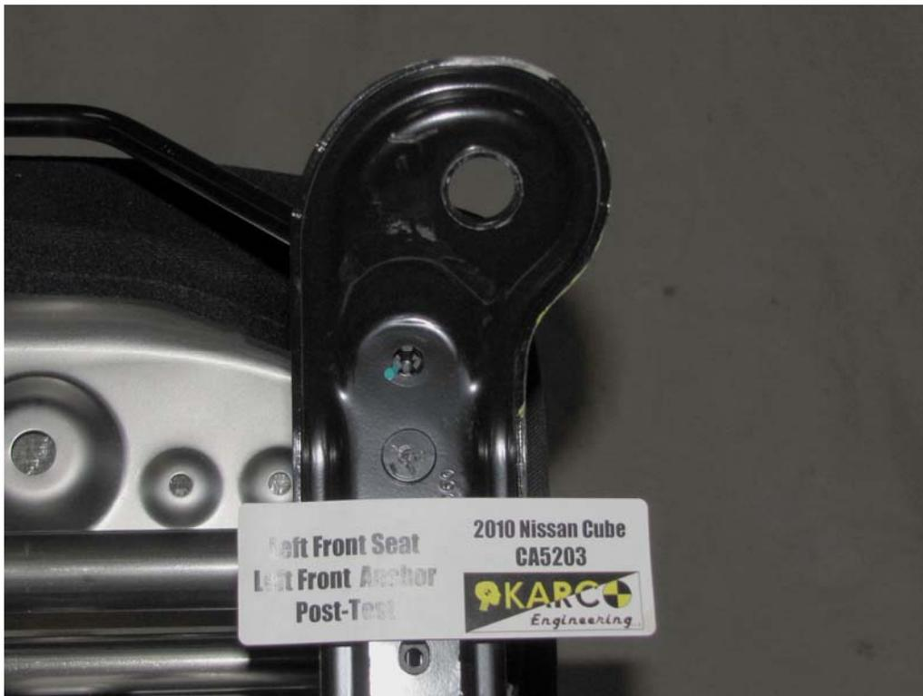
FIGURE 54. Seat Anchor, P1, Post-Test
