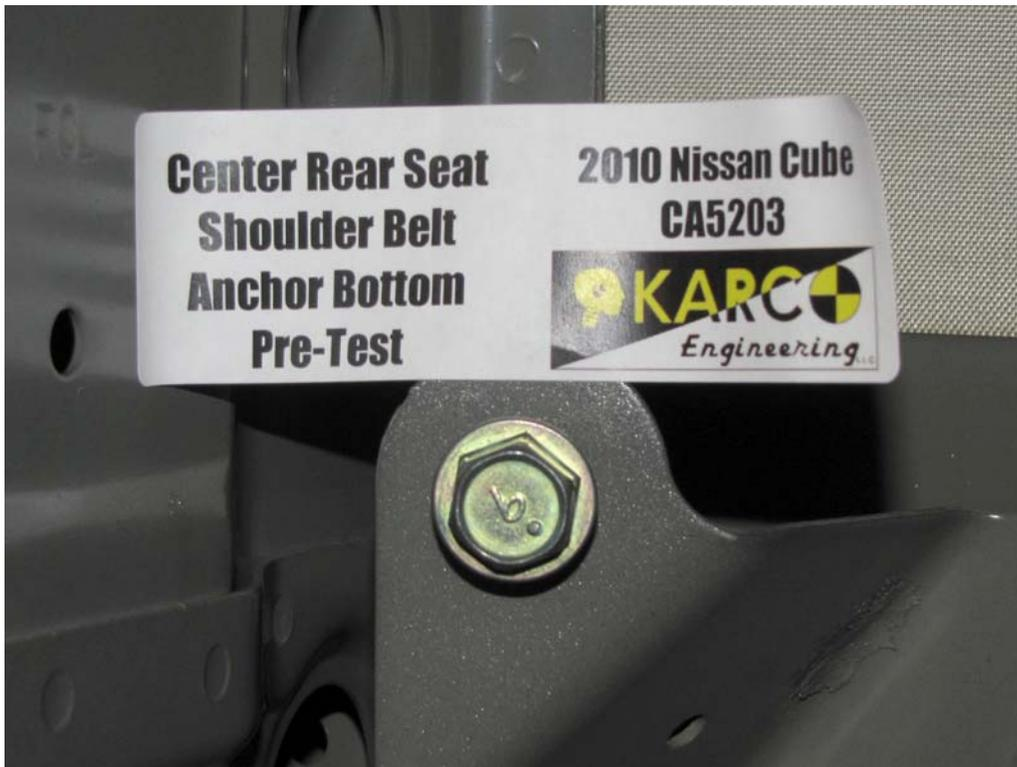
FIGURE 141. Shoulder Belt Anchor, P6, Pre-Test
