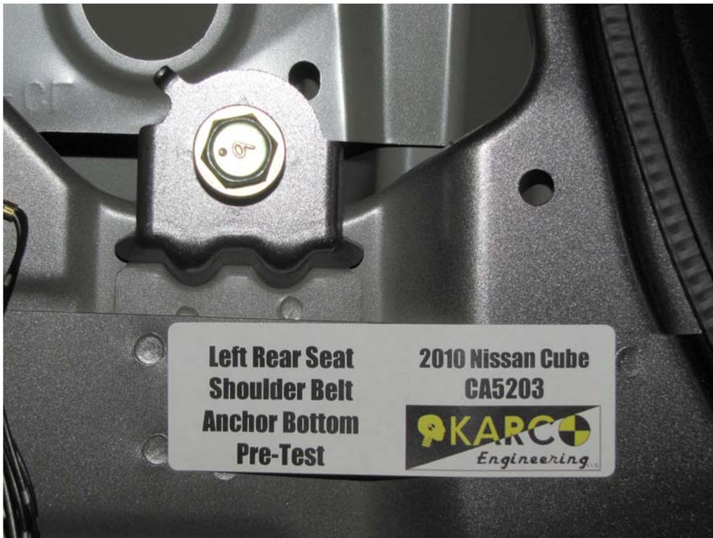
FIGURE 133. Shoulder Belt Anchor, P4, Pre-Test
