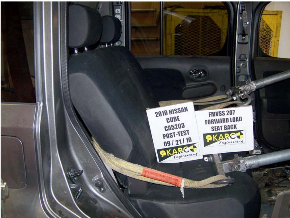
FIGURE 34. Forward Load on Seat Back, P3, Post-Test
