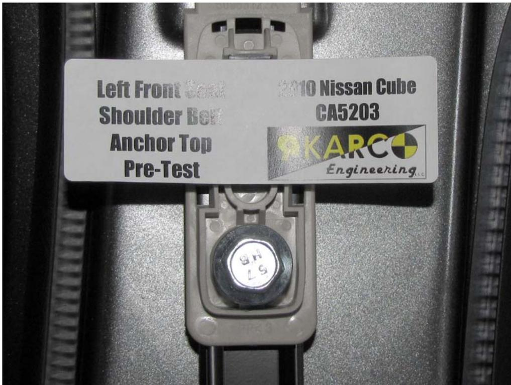
FIGURE 67. Shoulder Belt Anchor, P1, Pre-Test
