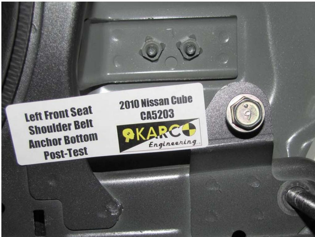
FIGURE 70. Shoulder Belt Anchor, P1, Post-Test
