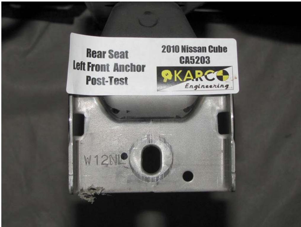
FIGURE 126. Seat Anchor, P4, Post-Test
