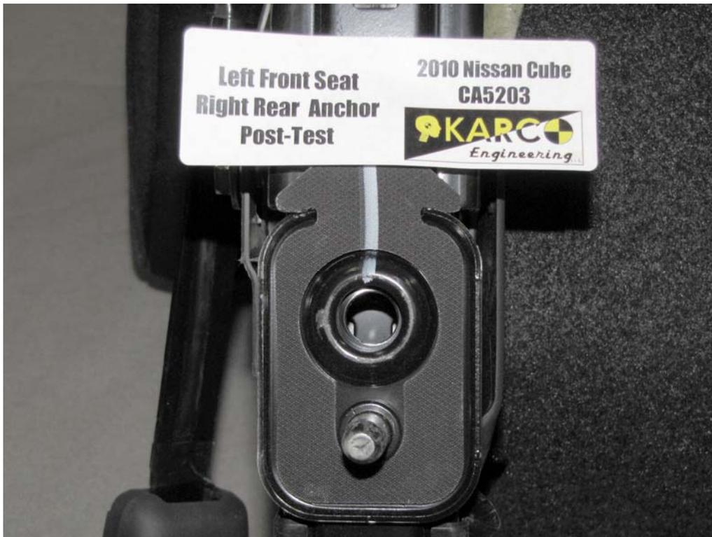
FIGURE 66. Seat Anchor, P1, Post-Test
