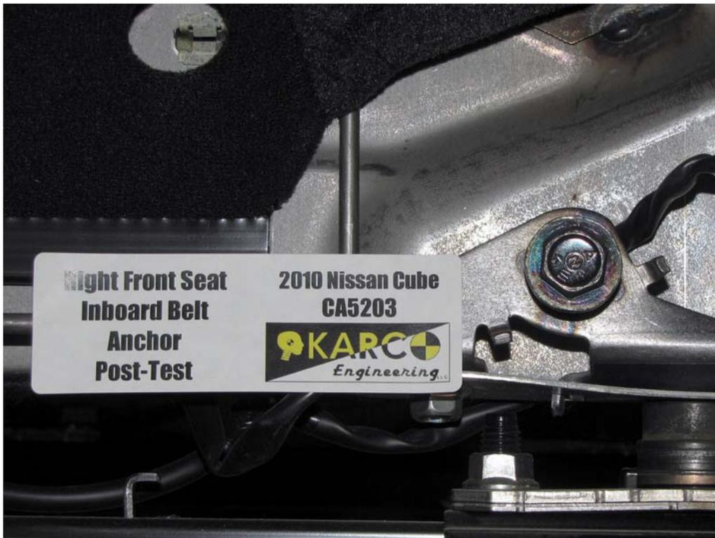
FIGURE 102. Belt Anchor, P2, Post-Test
