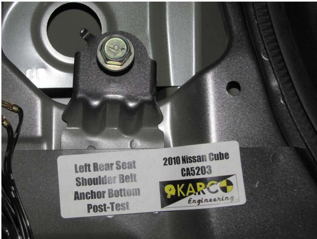
FIGURE 134. Shoulder Belt Anchor, P4, Post-Test
