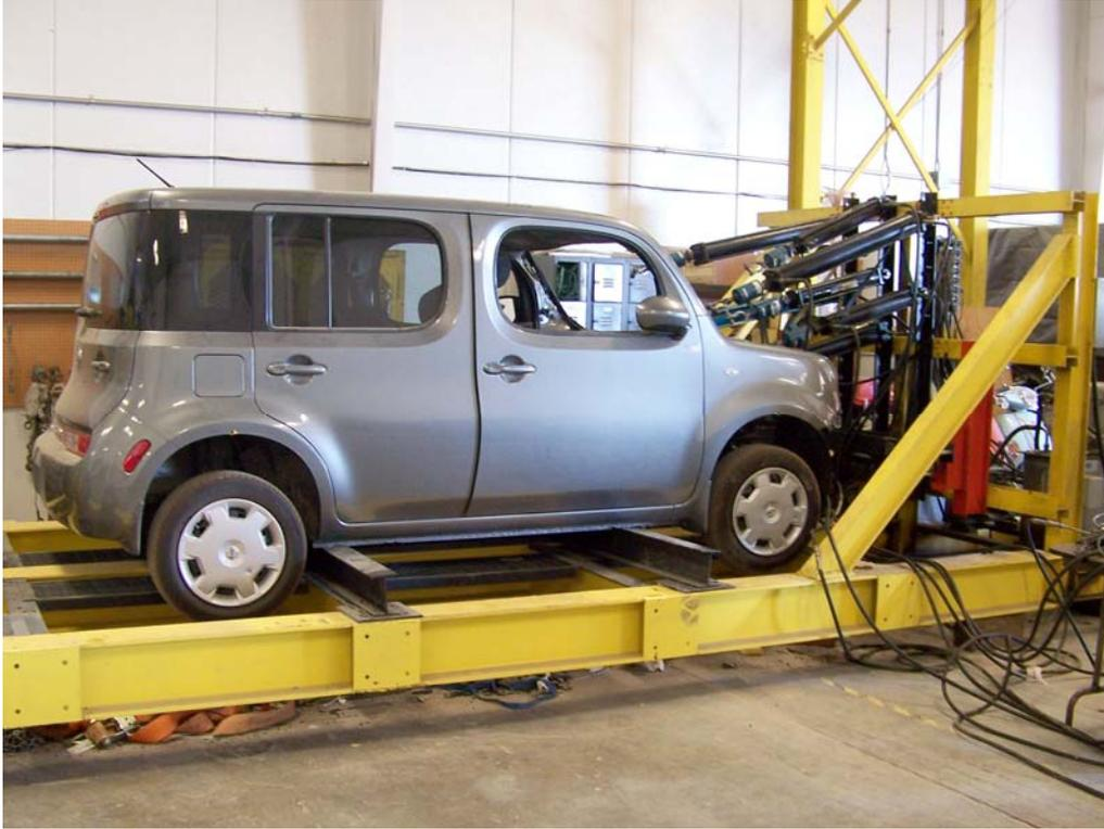
FIGURE 7. Vehicle Mounted in Test Fixture
