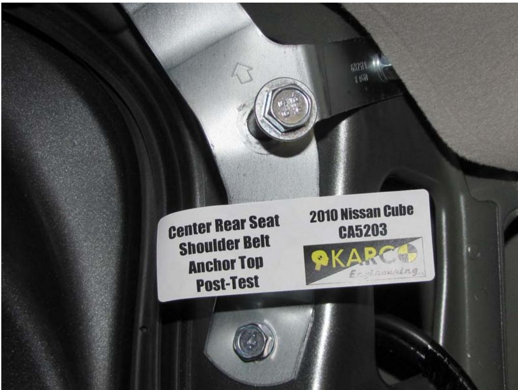
FIGURE 140. Shoulder Belt Anchor, P6, Post-Test
