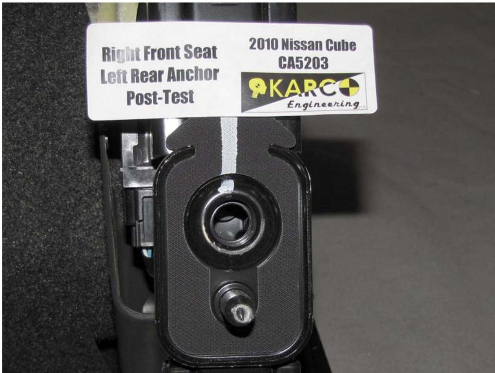
FIGURE 90. Seat Anchor, P2, Post-Test
