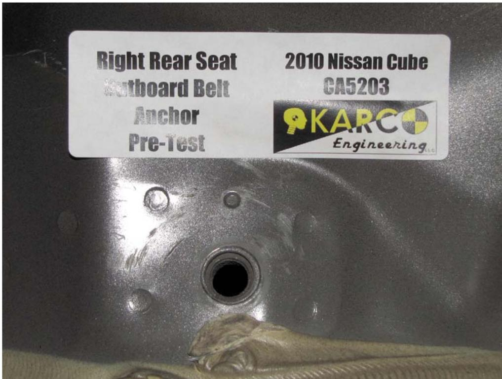
FIGURE 119. Belt Anchor, P3, Pre-Test
