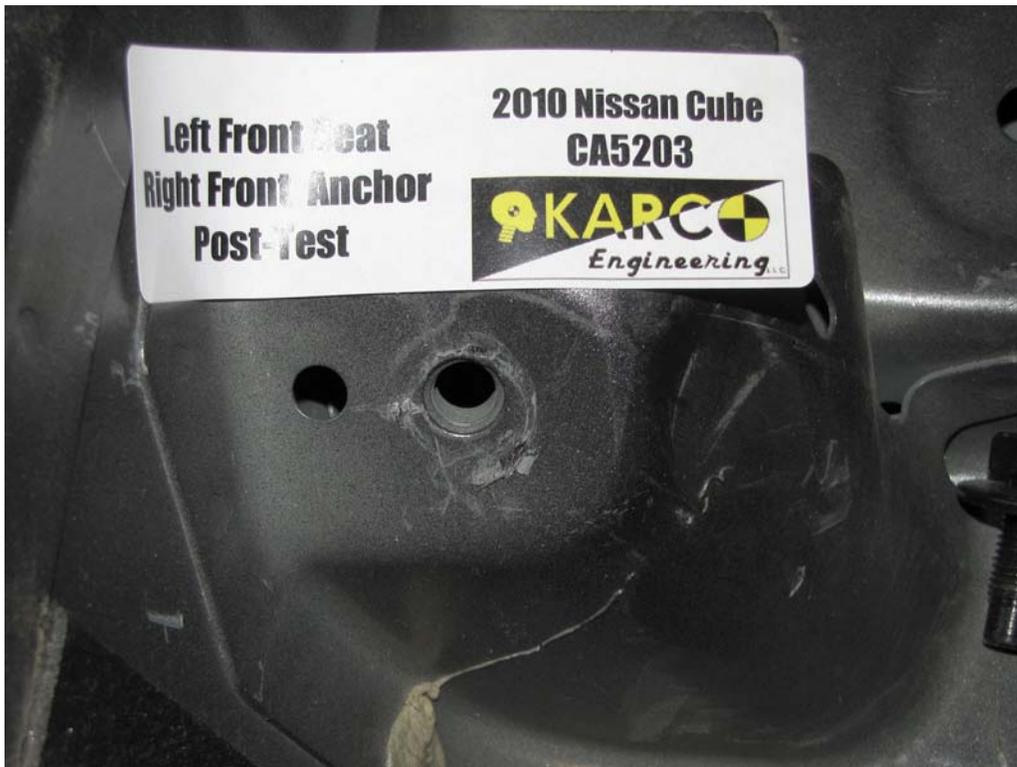
FIGURE 56. Floor Pan Anchor, P1, Post-Test
