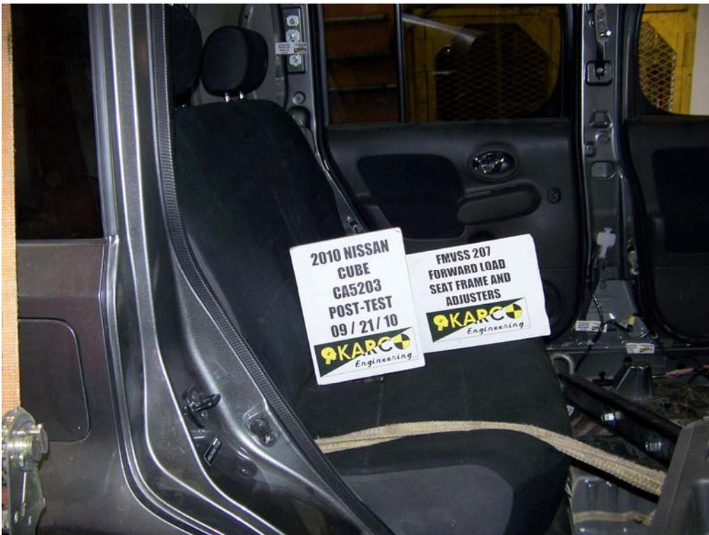
FIGURE 38. Forward Load on Seat Frame and Adjusters, P3, Post-Test
