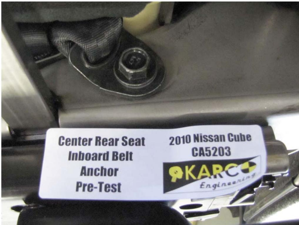
FIGURE 145. Shoulder Belt Anchor, P6, Pre-Test
