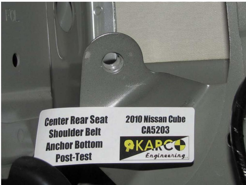
FIGURE 142. Shoulder Belt Anchor, P6, Post-Test
