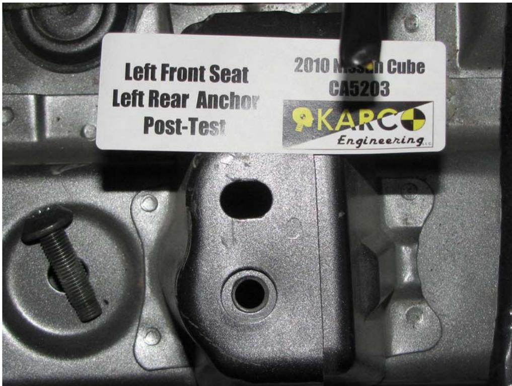
FIGURE 60. Floor Pan Anchor, P1, Post-Test
