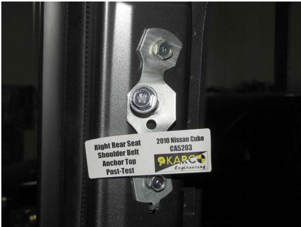
FIGURE 116. Belt Anchor, P3, Post-Test
