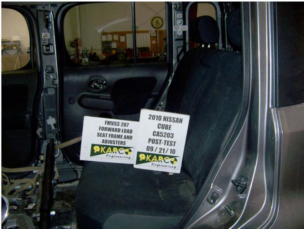
FIGURE 36. Forward Load on Seat Frame and Adjusters, P4, Post-Test
