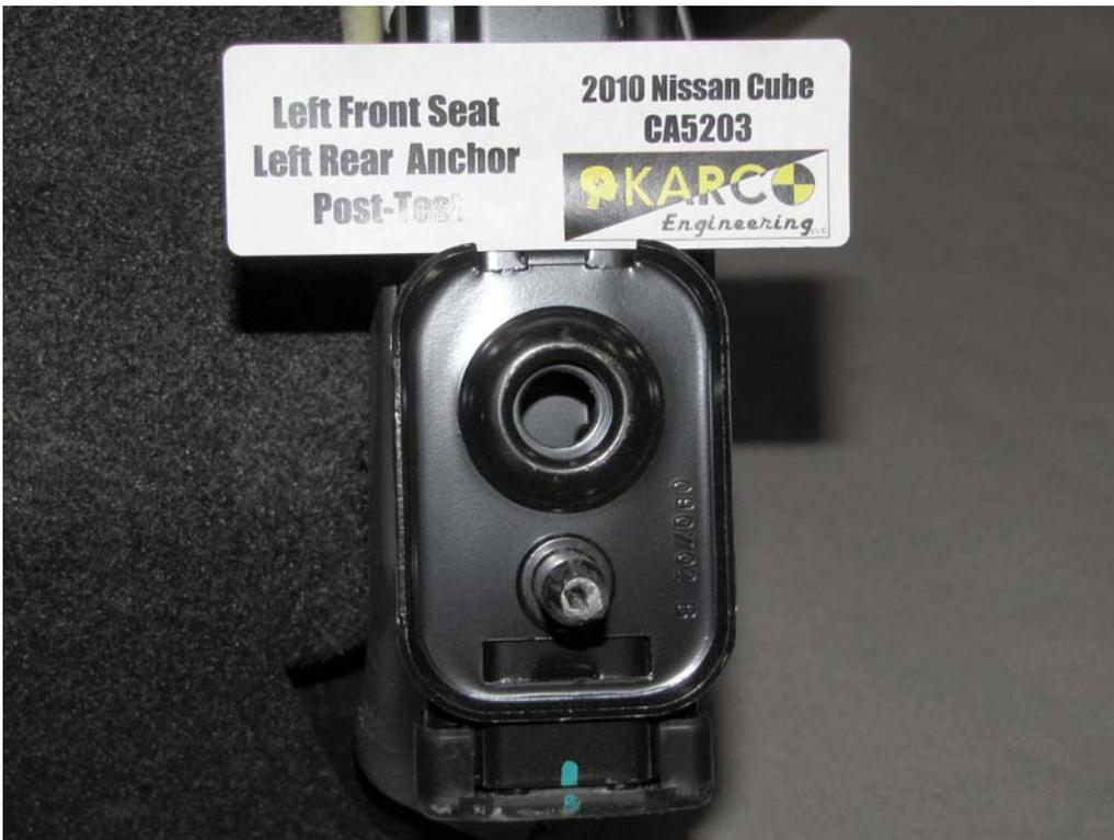
FIGURE 62. Seat Anchor, P1, Post-Test
