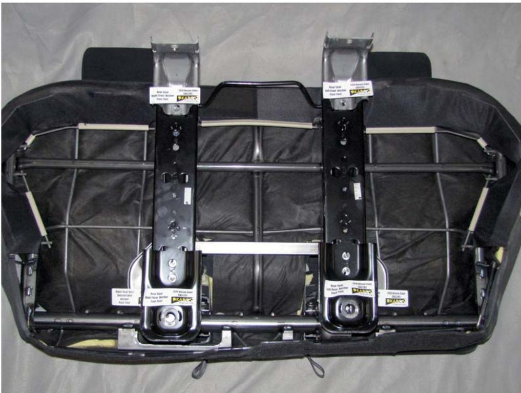
FIGURE 106. Seat Anchors, P3-P4-P6 Overall, Post-Test
