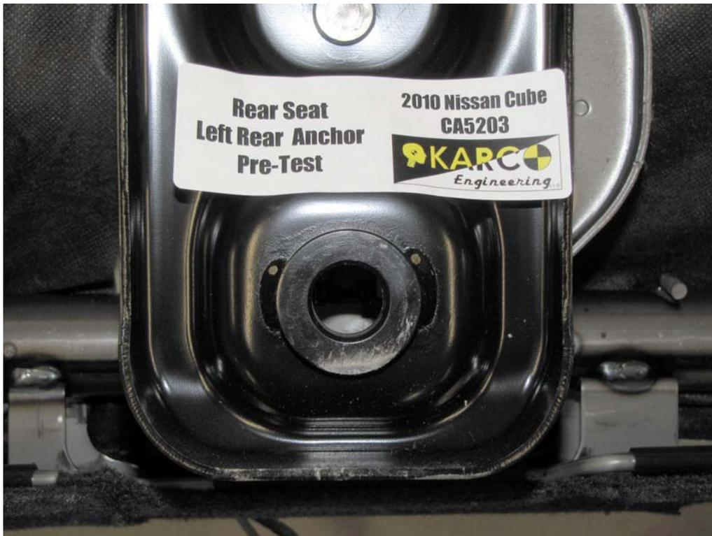
FIGURE 129. Seat Anchor, P4, Pre-Test
