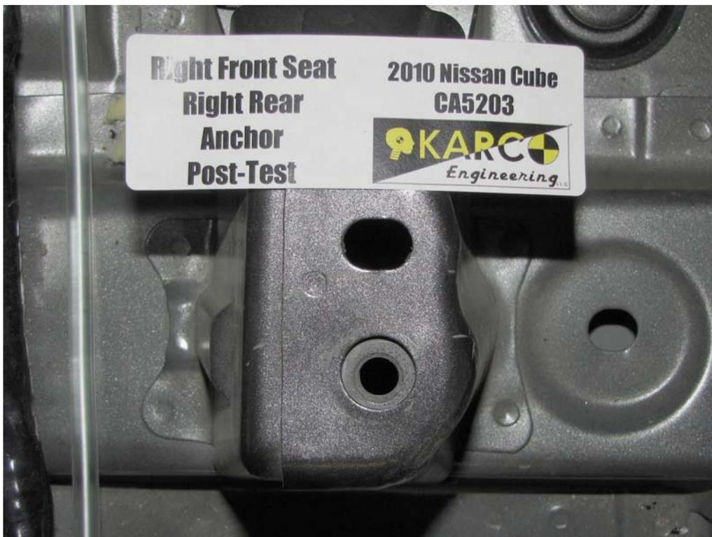
FIGURE 92. Floor Pan Anchor, P2, Post-Test
