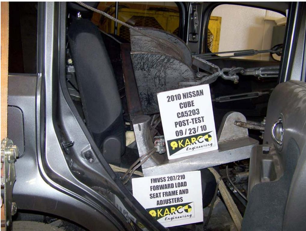
FIGURE 46. 207/210 Forward Load on Seat Frame and Adjusters, P3, Post-Test
