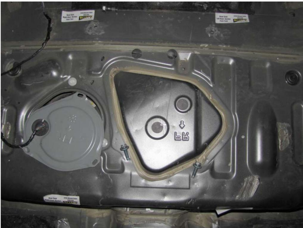
FIGURE 104. Floor Pan Anchors, P3-P4-P6 Overall, Post-Test
