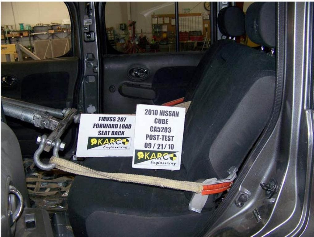
FIGURE 32. Forward Load on Seat Back, P4, Post-Test
