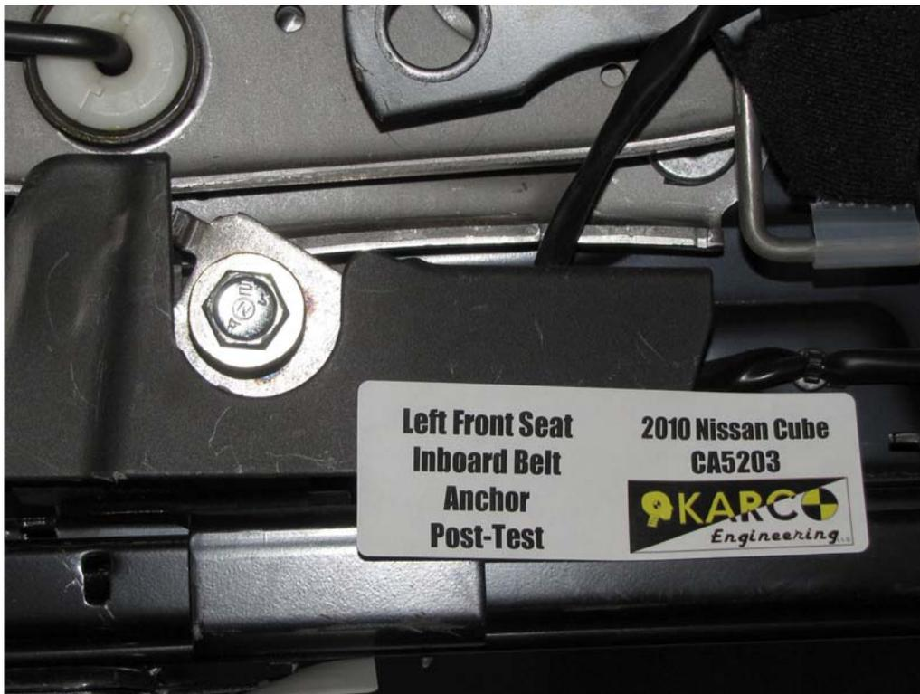
FIGURE 74. Belt Anchor, P1, Post-Test
