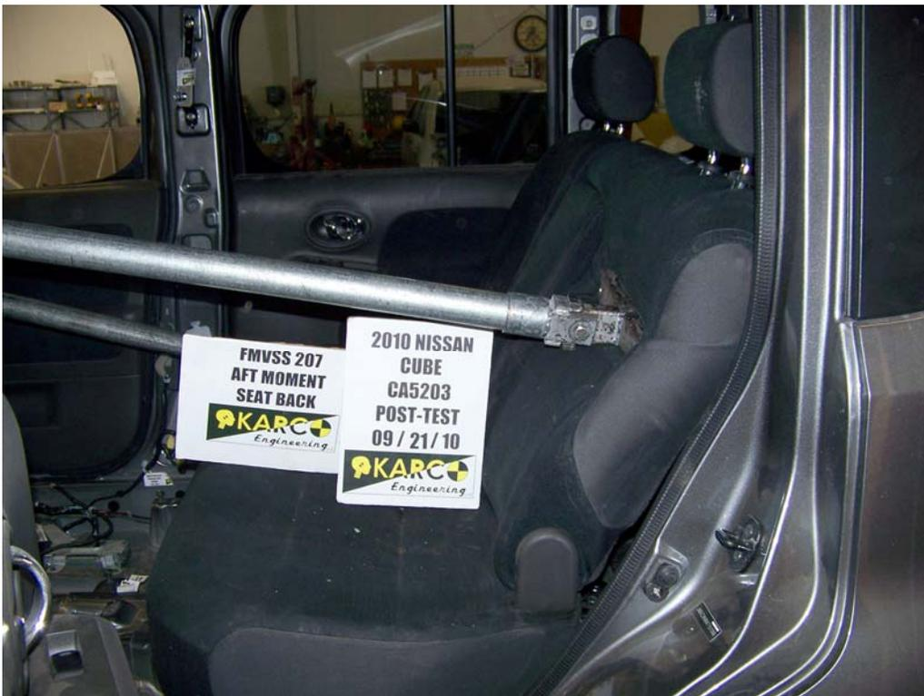
FIGURE 28. Aft Moment on Seat Back, P1, Post-Test
