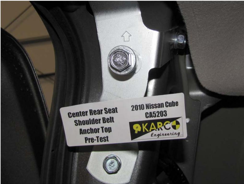
FIGURE 139. Shoulder Belt Anchor, P6, Pre-Test
