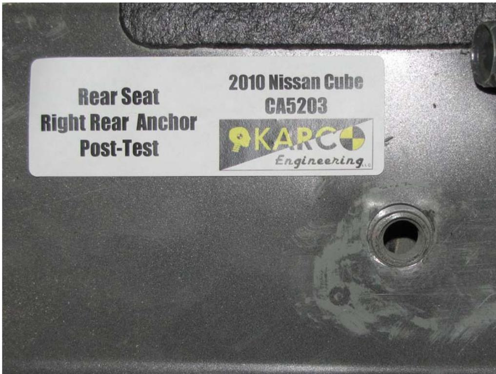
FIGURE 112. Floor Pan Anchor, P3, Post-Test
