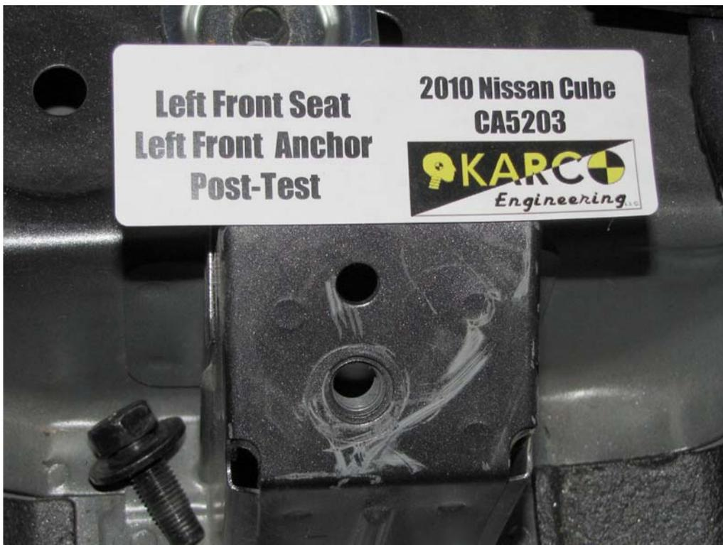
FIGURE 52. Floor Pan Anchor, P1, Post-Test
