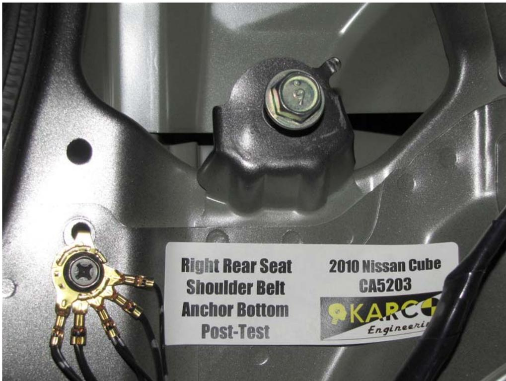
FIGURE 118. Belt Anchor, P3, Post-Test
