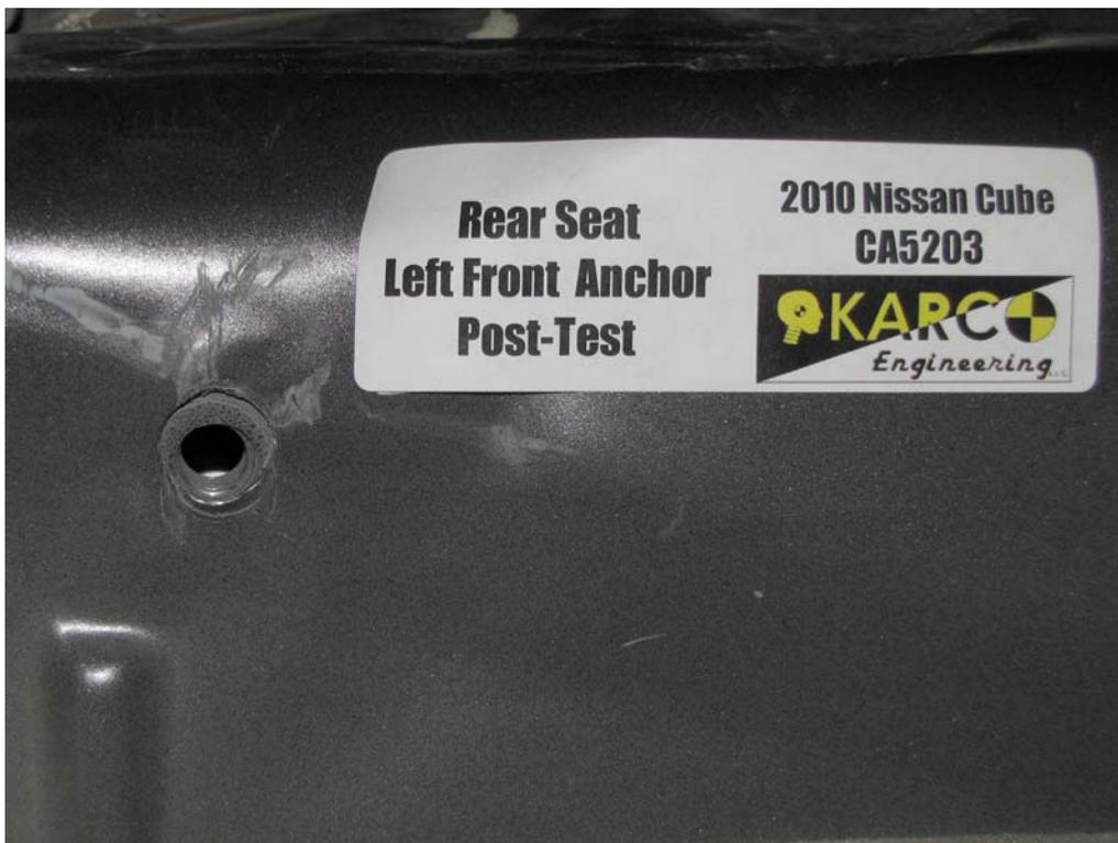
FIGURE 124. Floor Pan Anchor, P4, Post-Test
