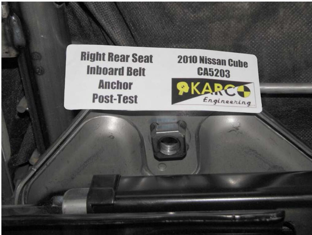
FIGURE 122. Belt Anchor, P3, Post-Test
