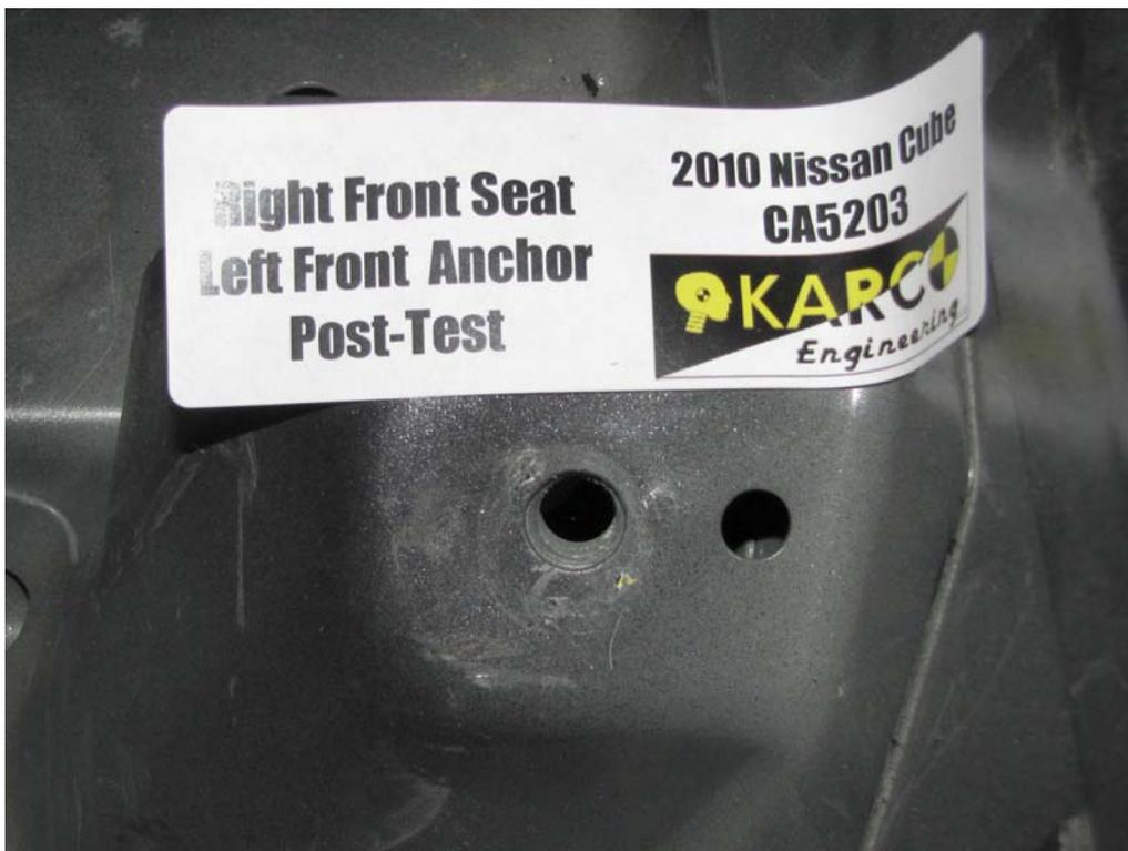
FIGURE 80. Floor Pan Anchor, P2, Post-Test
