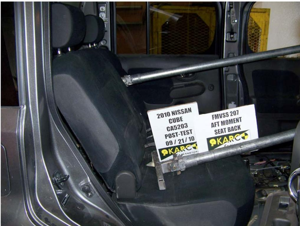
FIGURE 30. Aft Moment on Seat Back, P2, Post-Test
