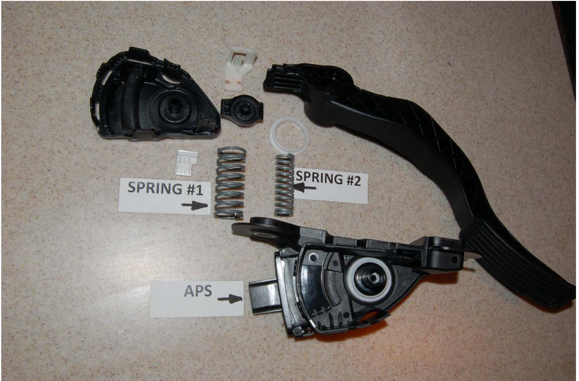
FIGURE 5.7 CLOSE-UP OF SPRINGS 1 & 2
