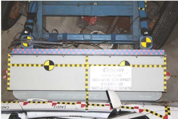
8 Overhead View of Aligned MDB and Vehicle at Impact Location
