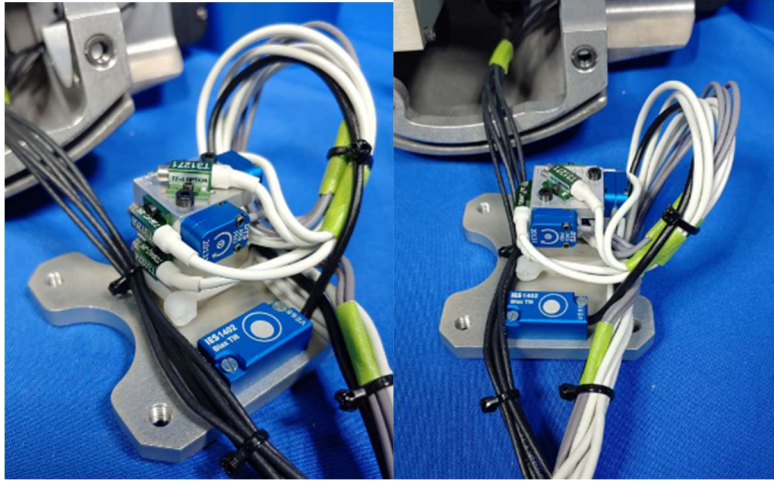
Figure 3-26. Head instrumentation wires strain relief
