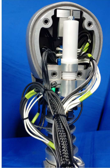
Figure 3-39. Routing cables for the head
