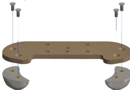
Figure 8-26. Remove the Left and Right Ischium Bones (474-45451,2) from the Ischium Bone Mount Plate (474-4542-A)
