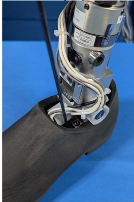
Figure 13-38. Foot wire bundle clearance during shoe installation
