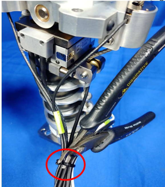
Figure 4-10. Remove the cable tie from the neck cable bundle
