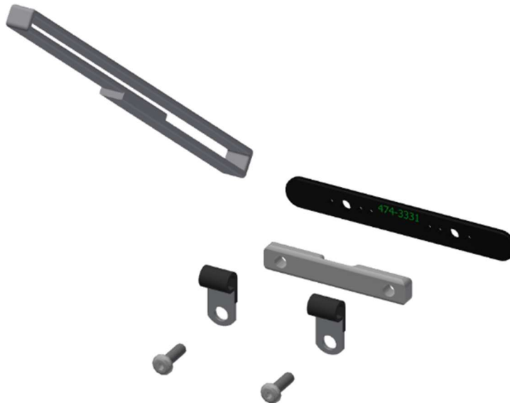
Figure 5-59. Install the Rib 1 Stiffener (474-3331), THOR Lifting Strap (472-3116), Lifting Strap Bracket (474-3025), and cable clamps (9003723)
