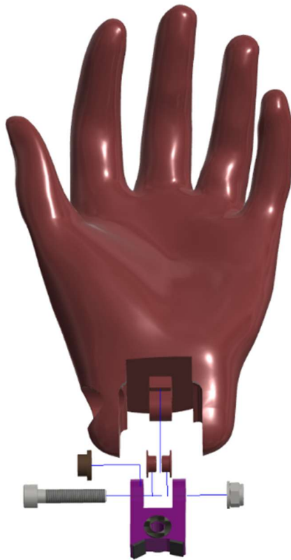
Figure 11-24. Install Wrist Rotator Clevis (474-6717-1,2) into Molded Hand (474-6900-1,2)
