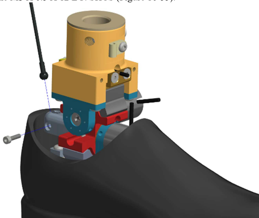
Figure 10-55. Attach the Achilles Cable to the Achilles Cable Retainer (474-5828)
