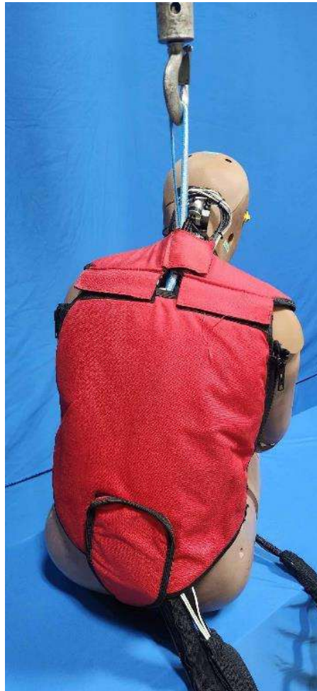
Figure 12-4. Lift dummy and install crotch strap
