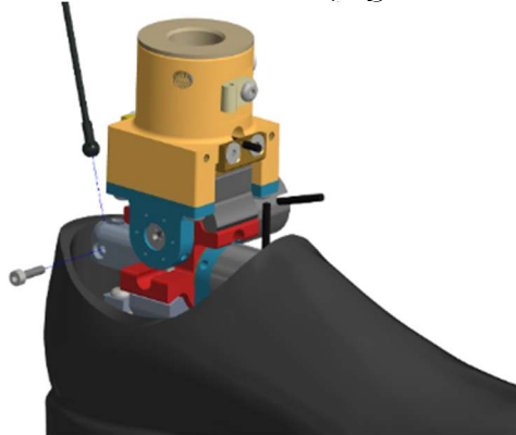
Figure 10-16. Remove the M3 Bolt in the Achilles Cable Retainer (474-5828)
