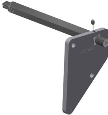
Figure 2-9. Tighten set screw into tool expander
