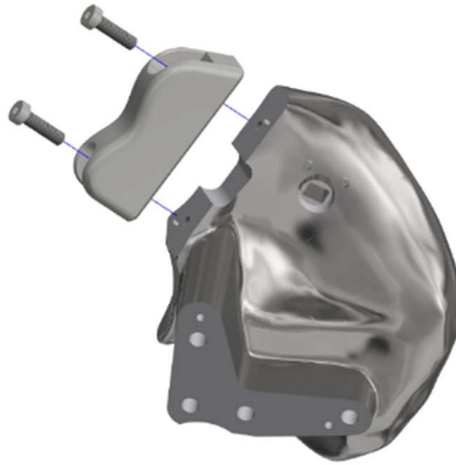
Figure 8-15. Remove the ASIS Load Cells from the Left and Right Iliac Wings (474-4540-1,2-A)
