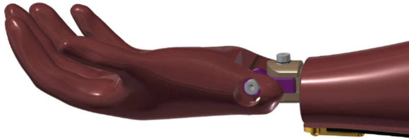
Figure 11-45. Wrist orientation for setting joint torque to 1G
