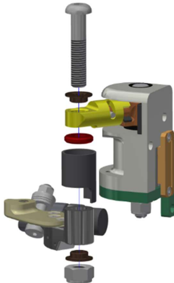
Figure 7-16. Connect the Lower Scapula (474-3505-1,2) to the Spine-Shoulder Coupler Assembly (474-3524-1,2-A)
