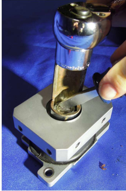
Figure 6-18. Remove the modified M12 Hex Lock Nut with a flat head screwdriver and a modified socket
