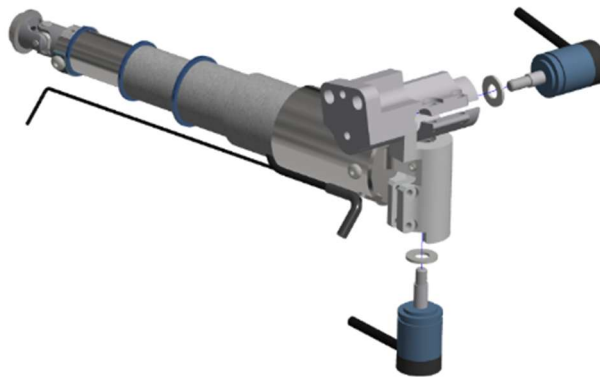
Figure 5-25. Remove potentiometers and washers from the assembly
