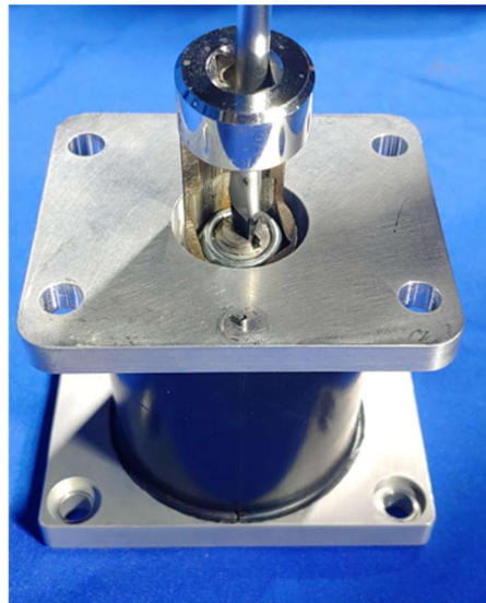
Figure 6-31. Install locknut to lumbar cable (474-3227)
