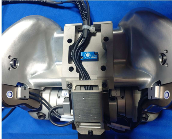
Figure 8-46. Strain relieve the instrumentation wires
