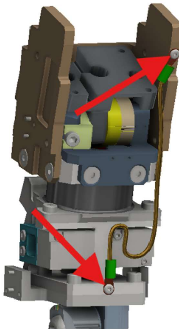
Figure 5-43. Attach the thorax ground cable
