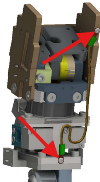
Figure 5-38. Remove the thorax ground cable
