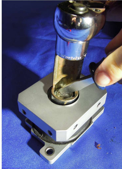
Figure 6-42. Install locknut to upper spine cable (474-3224)
