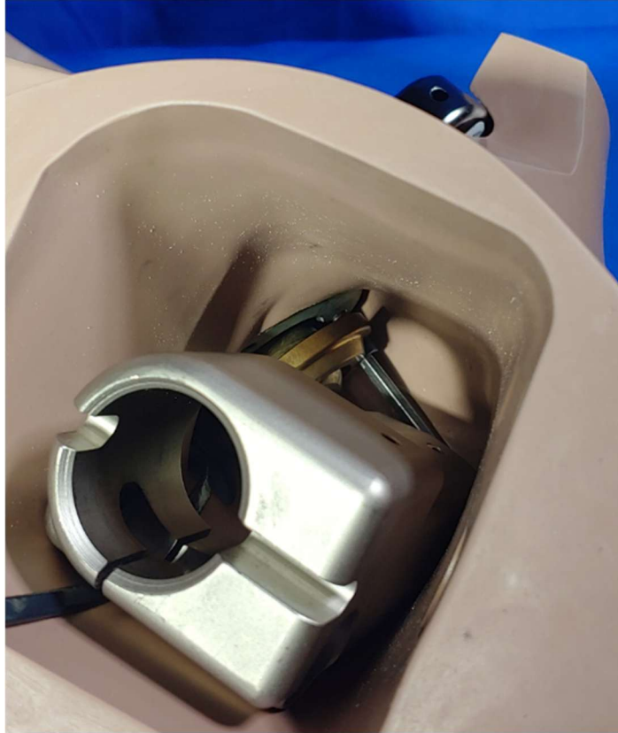
Figure 8-57. Accessing holes for installing femur assemblies
