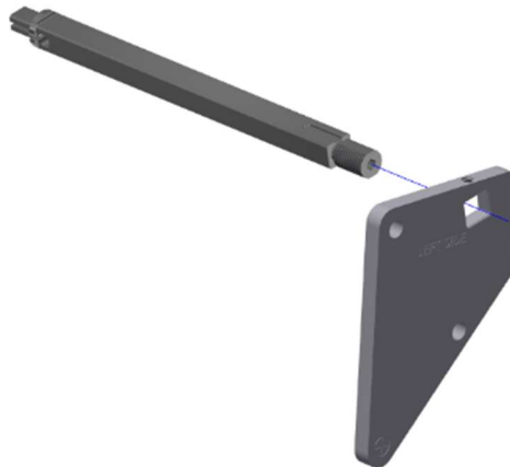
Figure 2-8. Install H-point tool expander into H-point tool plate
