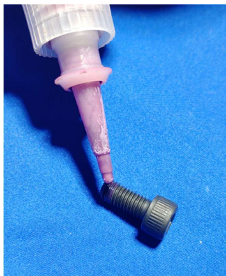
Figure 8-38. Apply Loctite to the M8 X 1.25 X 18 SHCS
