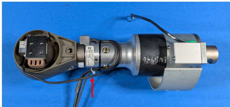
Figure 13-41. Knee slider wiring added to bundle and routed inside the leg (slider fully extended)
