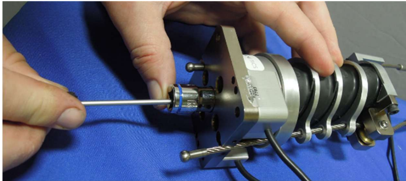
Figure 4-36. Install hardware for neck center cable
