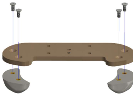
Figure 8-30. Install the Left and Right Ischium Bones (474-4545-1,2) to the Ischium Bone Mount Plate (474-4542-A)
