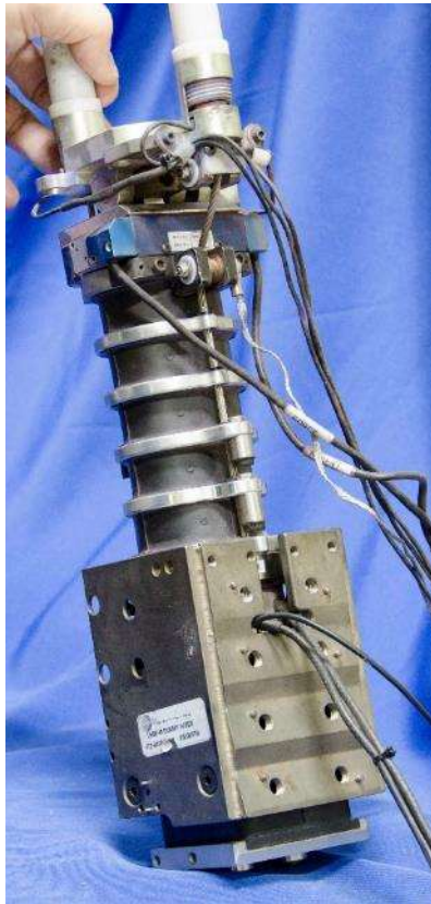
Figure 4-58. Routing wires for the lower neck load cell (SA572-S106).
