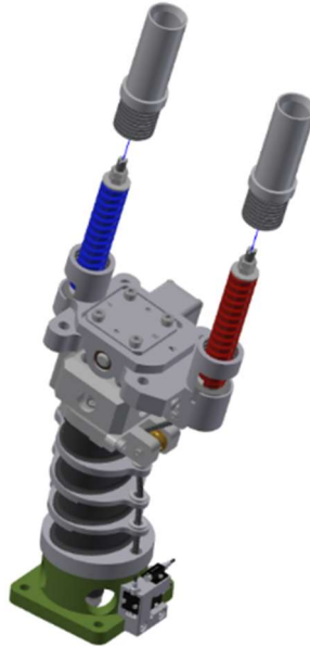
Figure 4-7. Unscrew the front and rear spring tubes (474-2303) from the head and neck mounting platform (474-2302-A)
