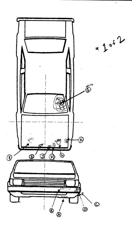
NOTES: Sketch all pedestrian contacts, include the size and depth in centimeters. Locate the pedestrian contacts from the intercept point of the centerline (lateral) and the front axles (longitudinal) in centimeters. Annotate observations which might be useful in reconstructing the accident (e.g., grass in tire bead, direction of striations, scuff on sidewalls, etc.).
