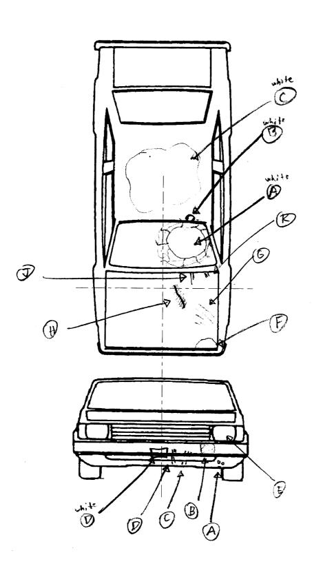
NOTES: Sketch all pedestrian contacts, include the size and depth in centimeters. Locate the pedestrian contacts from the intercept point of the centerline (lateral) and the front axles (longitudinal) in centimeters. Annotate observations which might be useful in reconstructing the accident (e.g., grass in tire bead, direction of striations, scuff on sidewalls, etc.).
