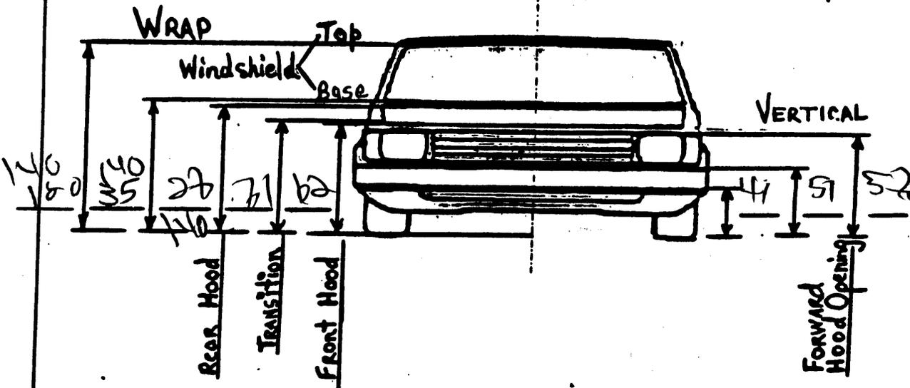
NOTES: Sketch all pedestrian contacts, include the size and depth in centimeters. Locate the pedestrian contacts from the intercept point of the centerline (lateral) and the front axle (longitudinal) in centimeters. Annotate observations which might be useful in reconstructing the accident (e.g., grass in the path, direction of slipstream, roof on sidewalks, etc.).
