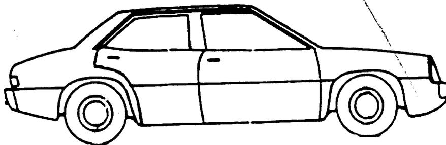
NOTES: Sketch all pedestrian contacts, include the size and depth in centimeters. Locate the pedestrian contacts from the intercept point of the centerline (lateral) and the front axes (longitudinal) in centimeters. Annotate observations which might be useful in reconstructing the accident (e.g., grass in tire bead, direction of striations, scuff on sidewalls, etc.).
