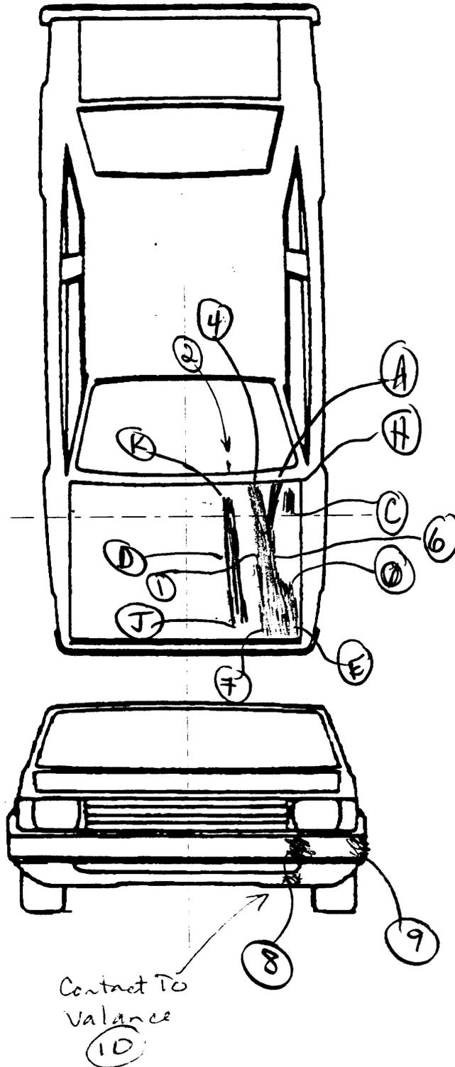
NOTES: Sketch all pedestrian contacts, include the size and depth in centimeters. Locate the pedestrian contacts from the intercept point of the centerline (lateral) and the front axles (longitudinal) in centimeters. Annotate observations which might be useful in reconstructing the accident (e.g., grass in tire bead, direction of striations, scuff on sidewalls, etc.).
