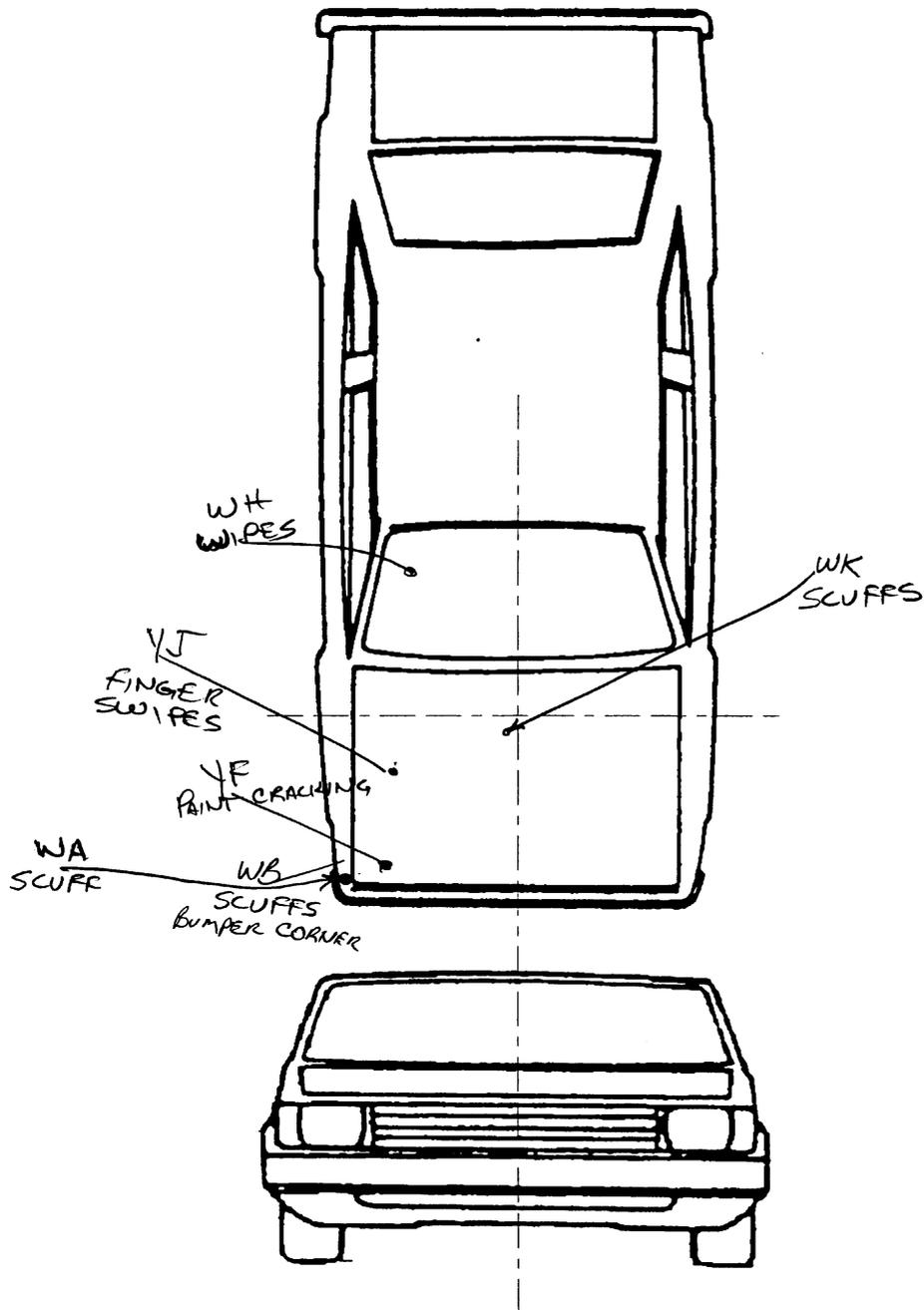
NOTES: Sketch all pedestrian contacts, include the size and depth in centimeters. Locate the pedestrian contacts from the intercept point of the centerline (lateral) and the front axes (longitudinal) in centimeters. Annotate observations which might be useful in reconstructing the accident (e.g., grass in tire bead, direction of striations, scuff on sidewalls, etc.).
