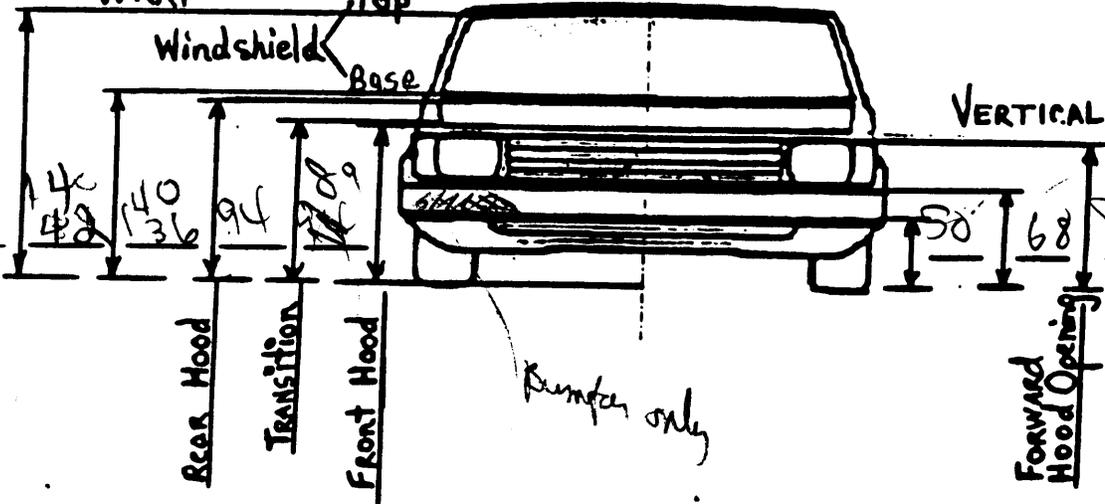
NOTES: Sketch all pedestrian contacts. Include the size and depth in centimeters. Locate the pedestrian contacts from the intercept point of the centerline (lateral) and the front axle (longitudinal) in centimeters. Annotate observations which might be useful in reconstructing the accident (e.g., grass in the back, direction of car, curb on sidewalk, etc.).
