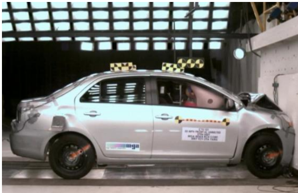
Figure 10 – Comparison of the global deformation for Yaris in NHTSA test no. 6069 and simulation
