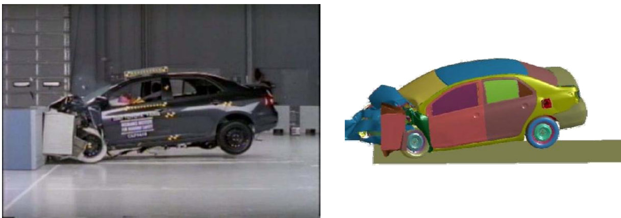
Figure 13 – Comparison of post-impact deformation of IIHS ODB test
