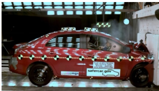
Figure 6 – Comparison of the global deformation for Yaris in NCAP Test 5677 and simulation
