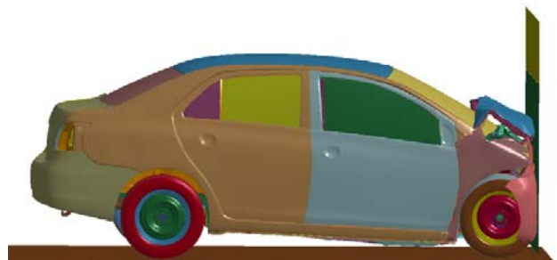
Figure 6 – Comparison of the global deformation for Yaris in NCAP Test 5677 and simulation
