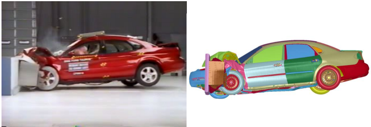
Figure 10 – Comparison of post-impact deformation of IIHS ODB test
