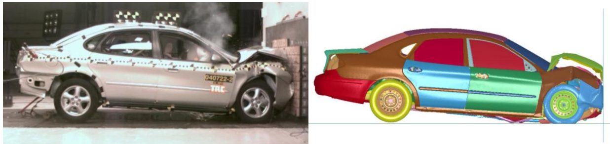
Figure 3 – Comparison of the global deformation for Taurus in NCAP test and simulation
