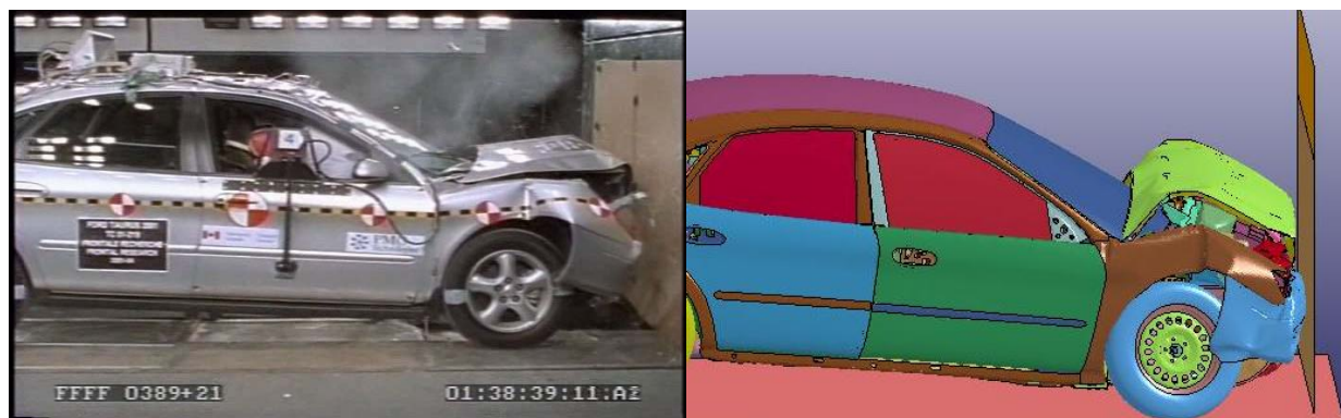
Figure 8 – Comparison of the global deformation for Taurus in 30 mph frontal test and simulation
