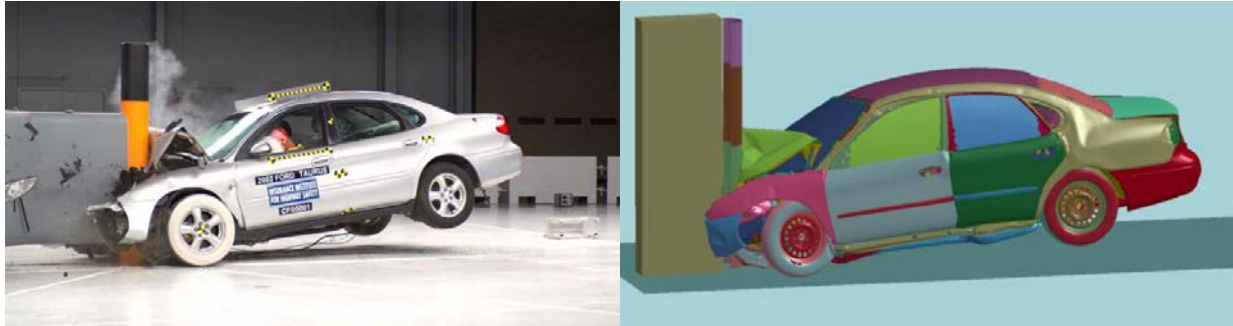
Figure 18 – Post-crash images of the Taurus in an offset rigid pole impact
