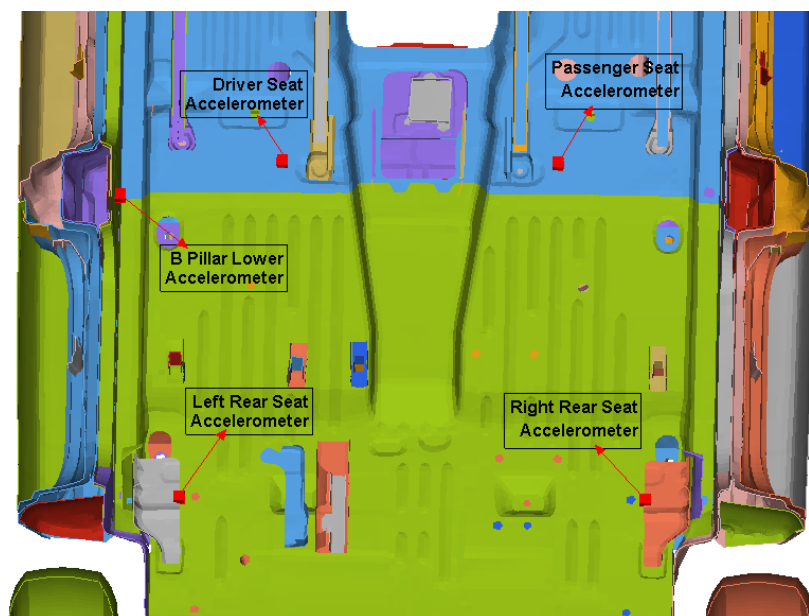
Figure 2 – Accelerometer locations in FE model
