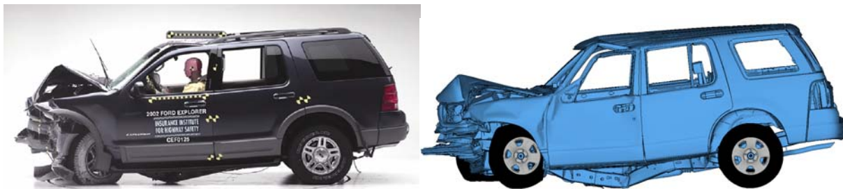
Figure 15 – Comparison of post-impact deformation for IIHS ODB test
