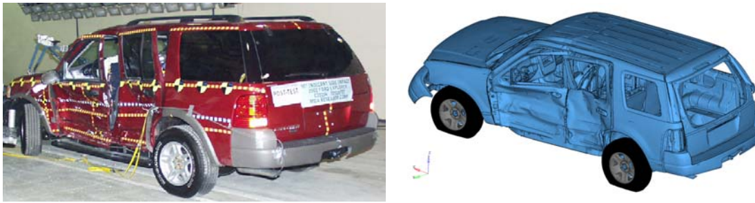
Figure 13 – Comparison of post-crash deformation between the side NCAP test and simulation
