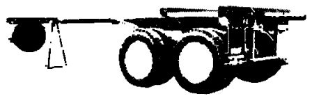
CONTRACTORS & UTILITIES DOUBLE BOLSTER TANDEM POLE TRAILER
