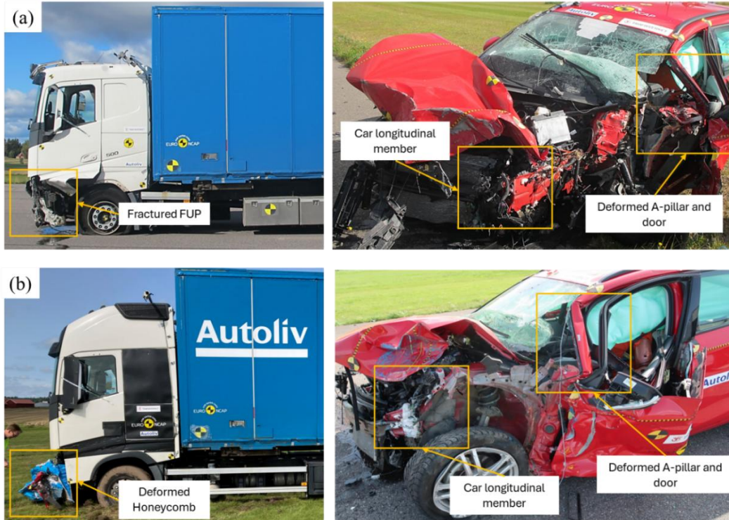
Figure 9: Deformed HGV and car structure in (a) Test-1 and (b) Test-2 after the frontal collision 50% offset impact between passenger car and HGV.
