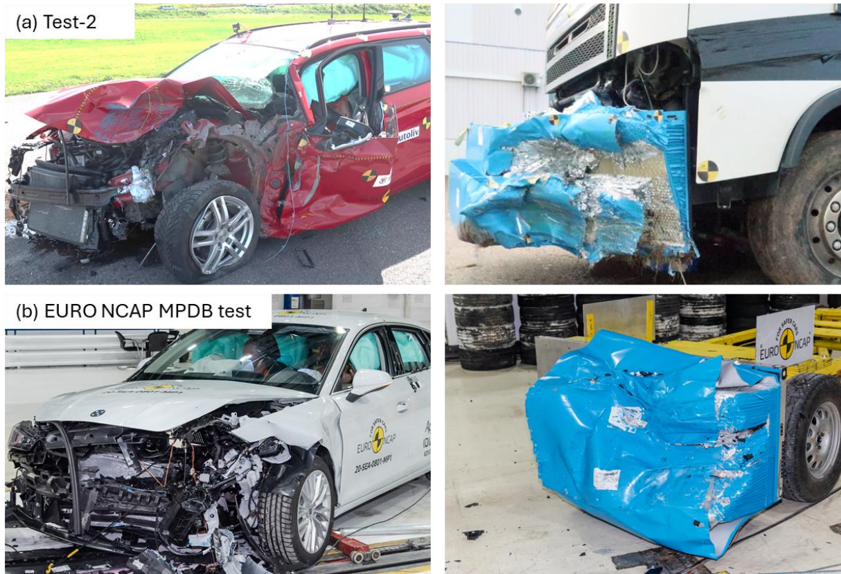
Figure 14: Deformation comparison for the car in the 50% offset frontal impact between (a) Test-2 (Passenger car and HGV), (b) car to MPDB in EURO NCAP test.
