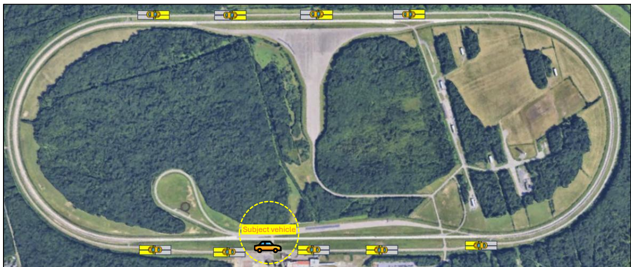
Figure 1. A 6.9 km private track was used for on-road testing. Nine target vehicles were placed around the track as indicated by the pin icons on the figure. Subject vehicle starting position remains the same for all laps.
