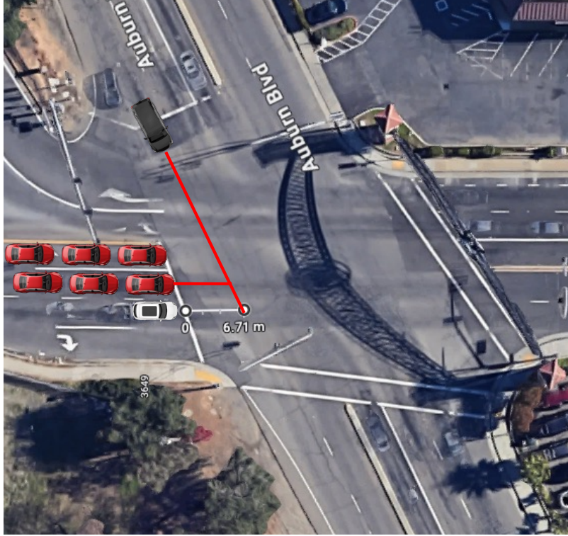
Figure 3: Three-vehicle collision ID 396273543, at the signalized intersection of Fulton Ave and Auburn Blvd in Sacramento, California, is an instance of car-to-car crossing, straight crossing paths (CCCscp), near side, tightly obstructed. The black vehicle runs a red light, while the white vehicle and one of the red ones start driving from the stop line.
