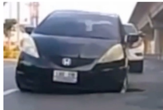
(e) Collision with open manhole
