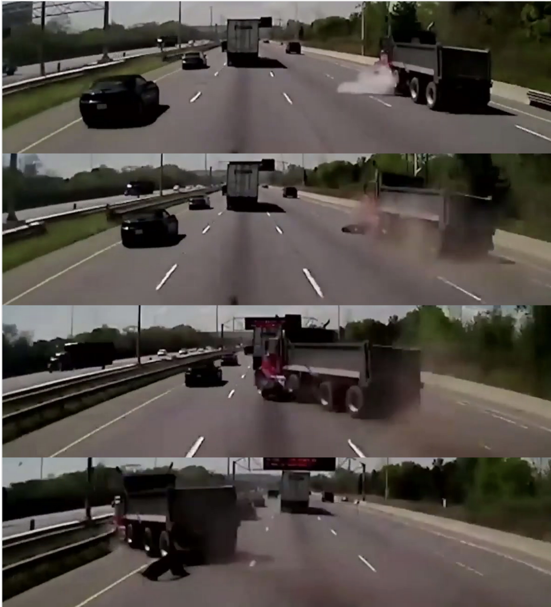
Figure 4: Keyframes of dashcam video showing tire blowout, vehicle losing control, and veering into opposite traffic.
