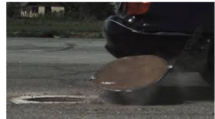
(c) Vehicle dislodging manhole cover
