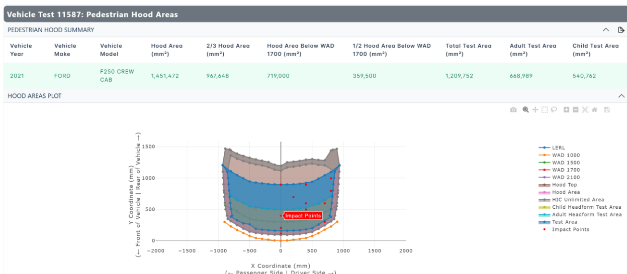
Figure 14. Sample pedestrian hood analysis results generated by WebSAT.
