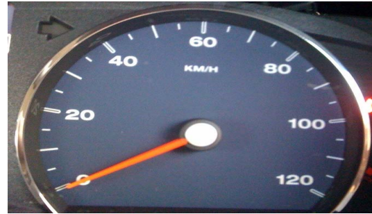
Figure 2. Reconfigured speedometer showing top speed of 120km/h
