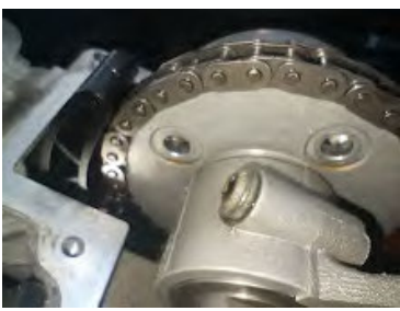
4) intake vanos gear (all 4 bolts are broken).jpg 490K
