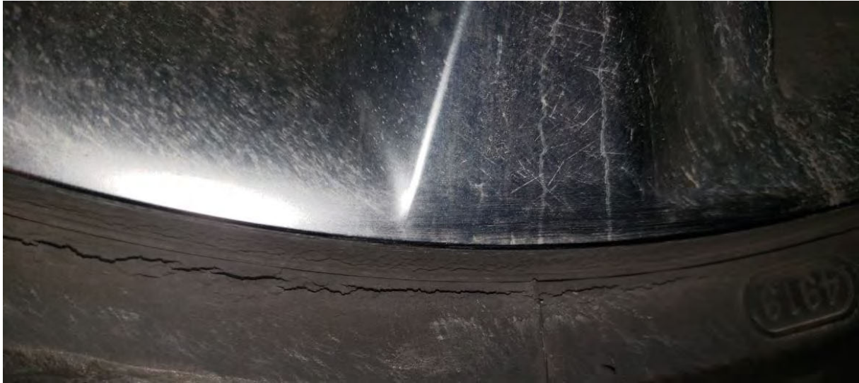
Picture 4 (Similar or more worse cracks on the all 4 tires)
