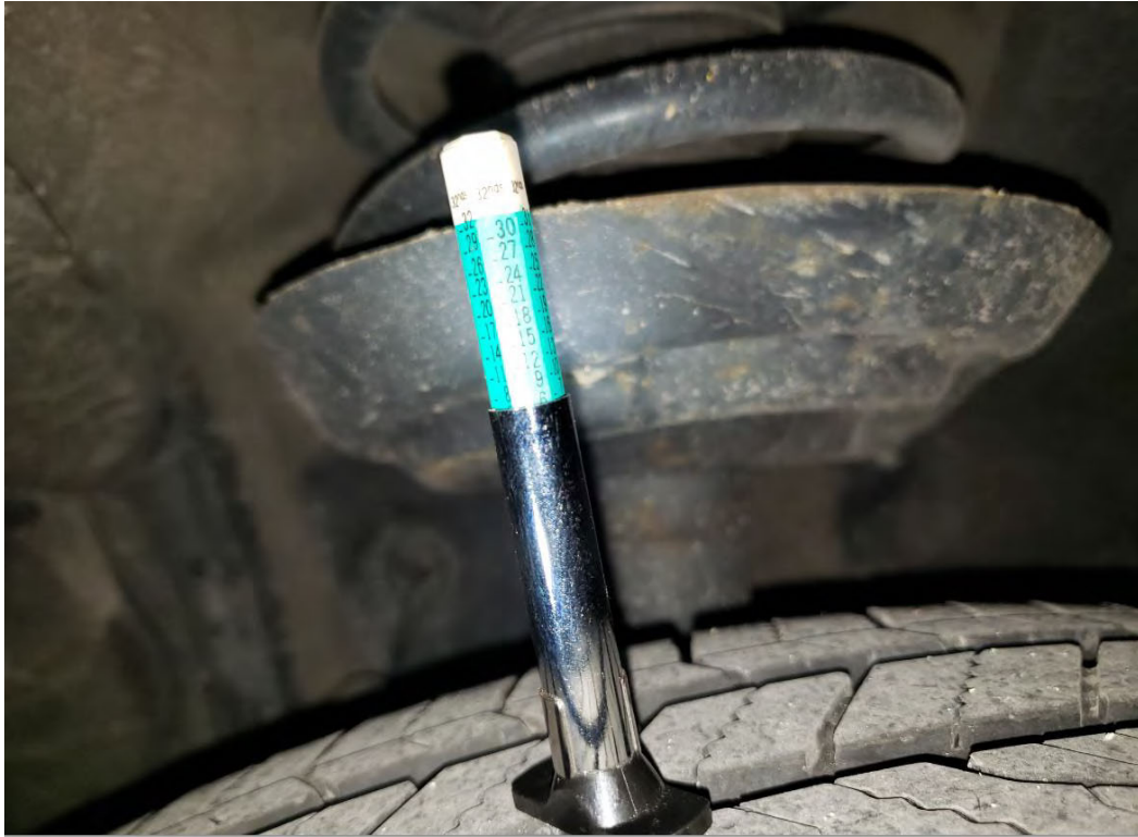
Picture 5 (tires had deepness on the track between 6/32 and 8/32)
