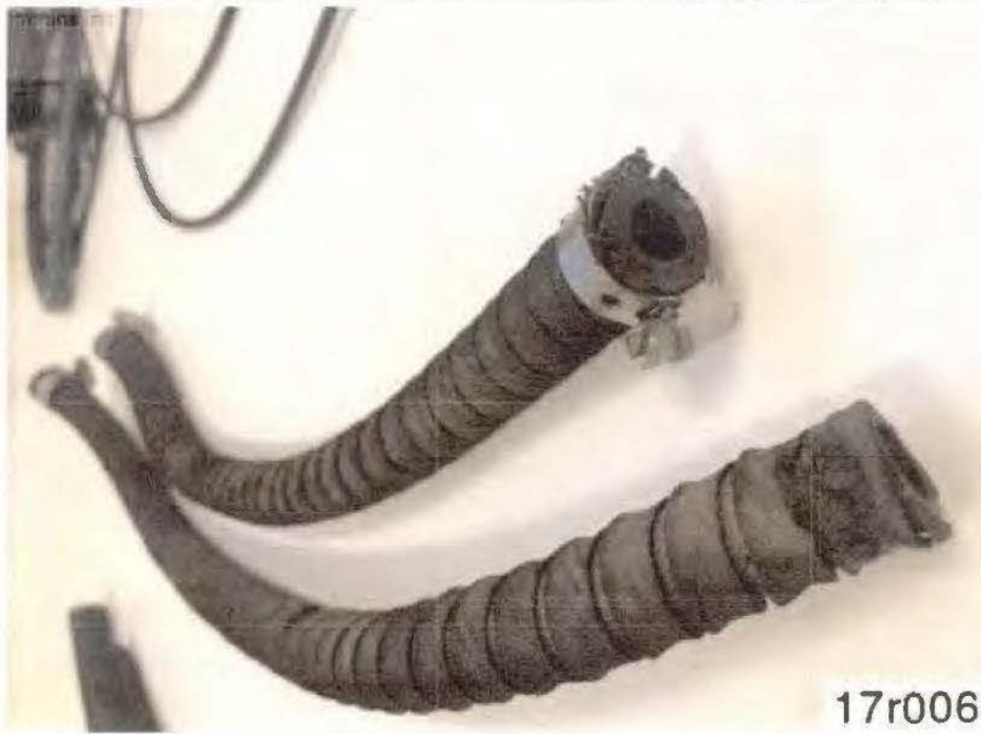
Figure 2, Old LP Fuel Hoses that are Susceptible to Cracking
