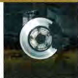
Damaged brake rotor from metal-to-metal contact
