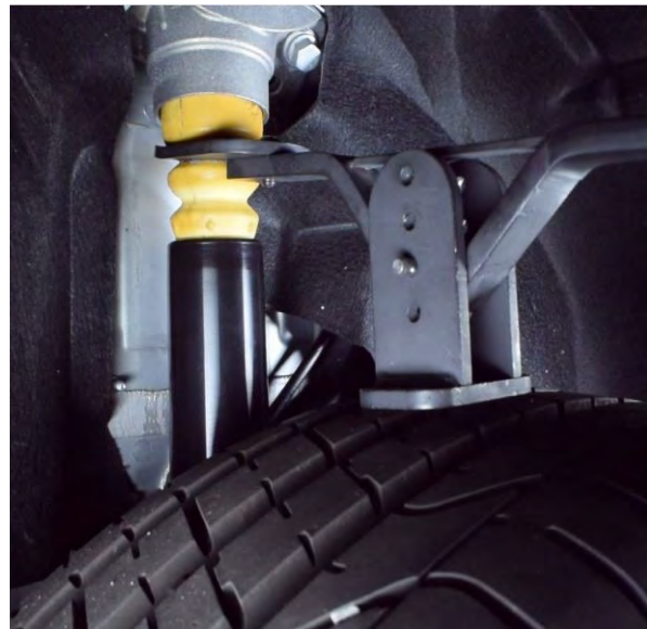
Figure 2. The SET900 tool being used to install a rear bump stop.
