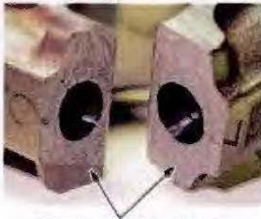
The uneven mating surfaces are uniquely matched and not interchangeable.
