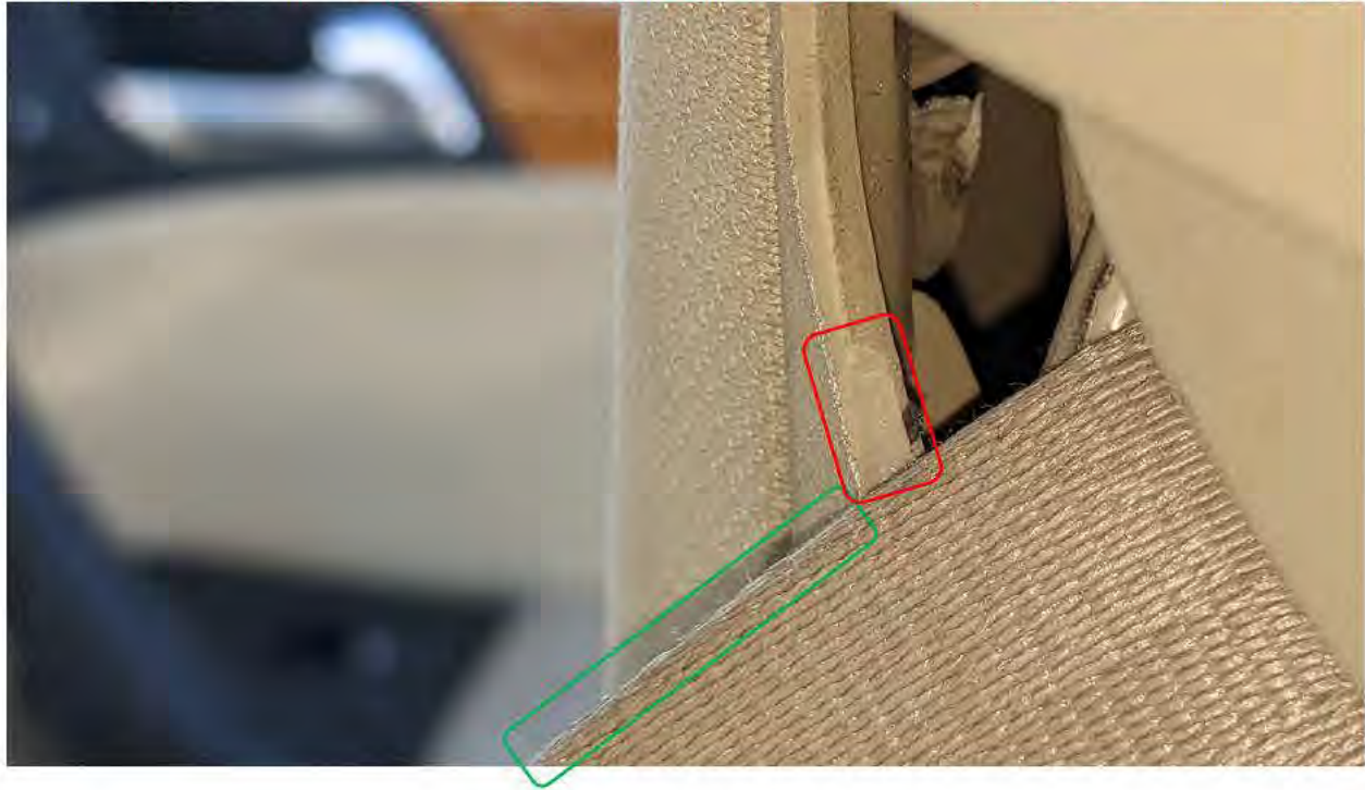
Front Passenger's Seatbelt. Red: Plastic Melting on B-Pillar Trim Green: Frayed Edge of Seatbelt Webbing
