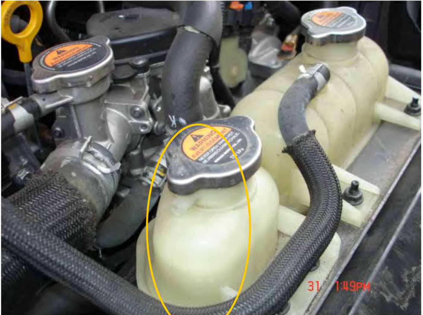
Heat exchanger coolant reservoir is empty
