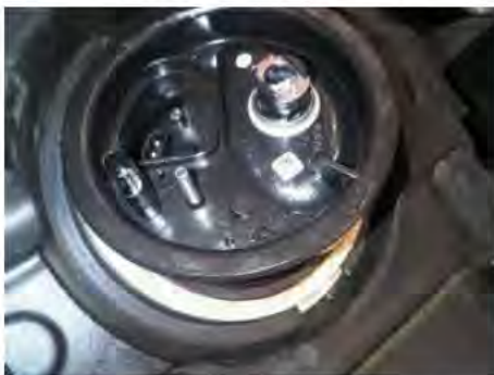
K1200S New Fuel Pump Unit - Metal Reinforcing Ring on Base Plate Boss
