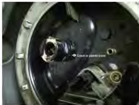
K1200S Fuel Pump-Unit Base cracked
