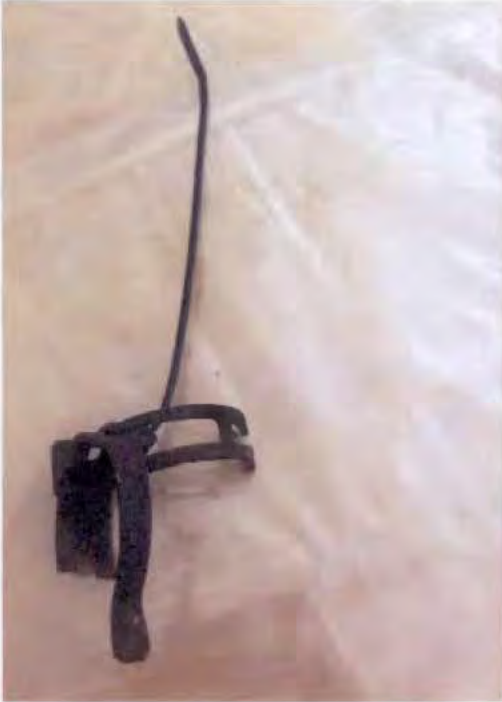
Pictures of corroded radiator clamp:
