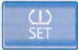
Fig. 99 In the glove compartment: SET button for the Tire Pressure Monitoring System.
