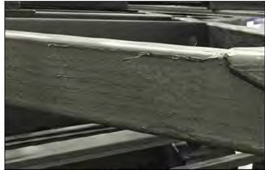
Figure 11 Runs and build-up
