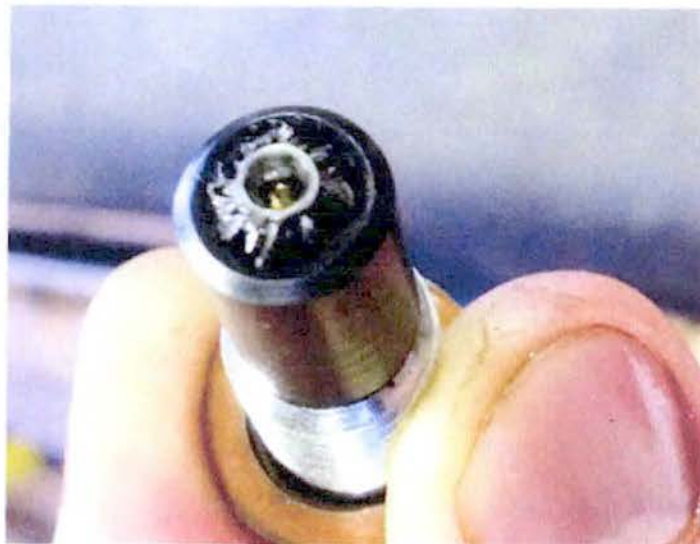
FIGURE 3: Photo of magnetic plug taken after cleaning off external metal shards and then 'pumping' magnet on plug's shaft; exposing additional metal shards and debris trapped inside magnet's core.
