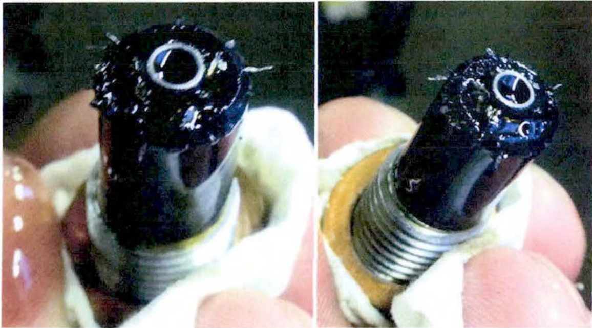
FIGURES 1 & 2: Photos of magnetic plug taken immediately after removal from engine showing numerous metallic shards and debris.
