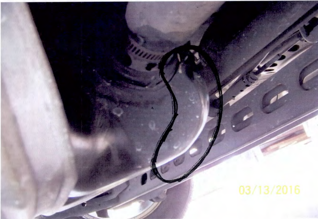
Gasoline leaks by the tank inlet
