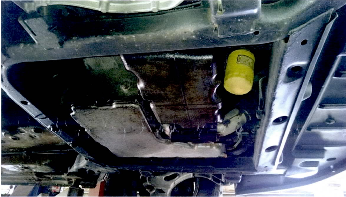
Picture 1: Side view under the 1999 Cadillac Seville STS model. Oil leak onto the exhaust manifold.
