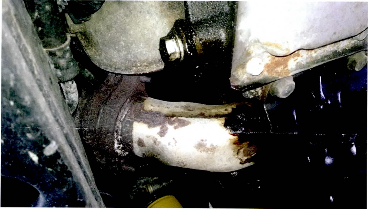
Picture 3: Side view under the 1999 Cadillac Seville STS model. Oil leak onto the exhaust manifold.
