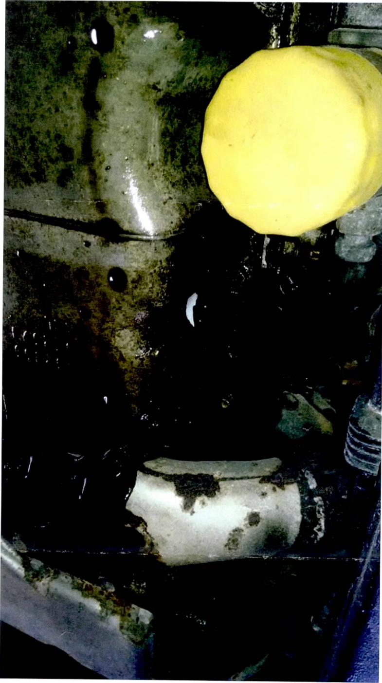
Picture 2: Side view under the 1999 Cadillac Seville STS model. Oil leak onto the exhaust manifold.
