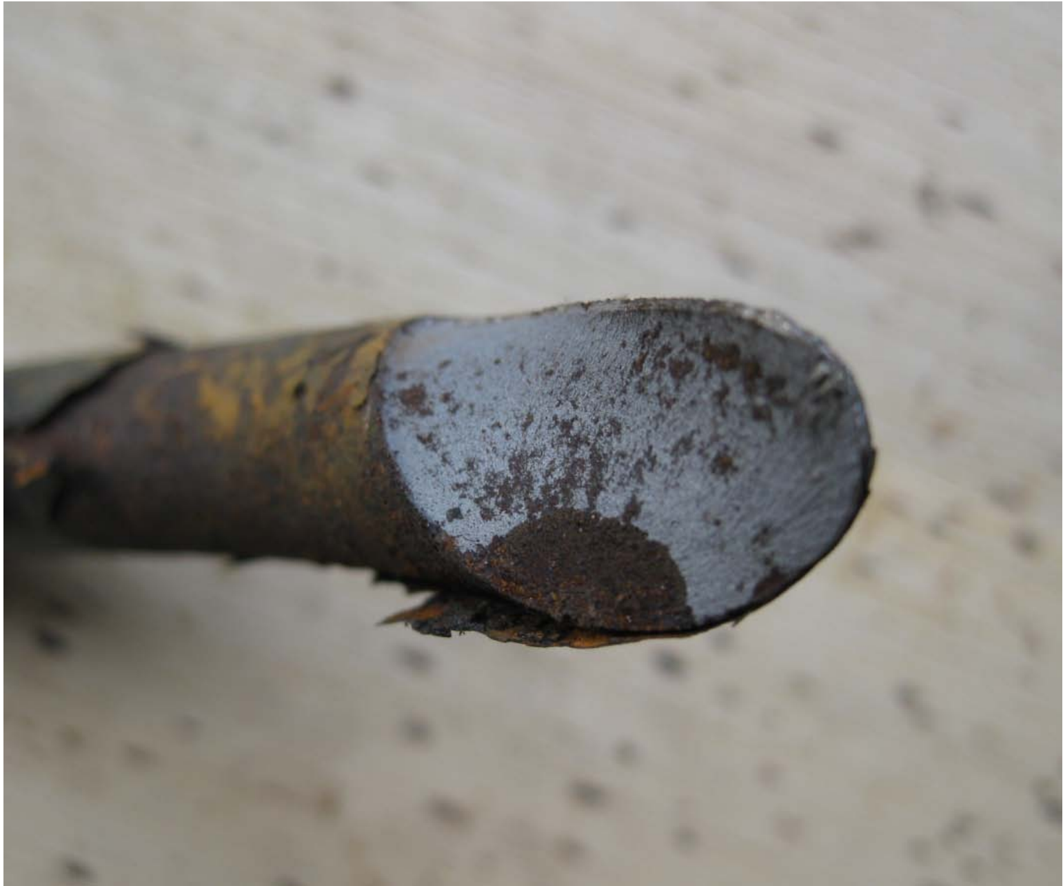
CLOSEUP OF BROKEN (FAILED REGION) OF SMALLER SIDE BROKEN SPRING
