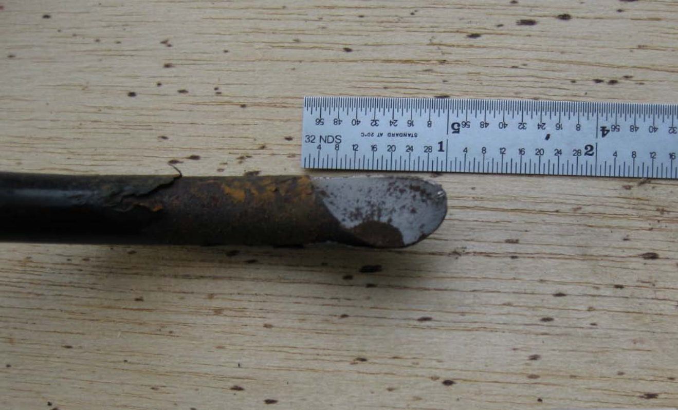
CLOSEUP OF BROKEN AREA FROM SMALLER PIECE OF BROKEN SPRING.
