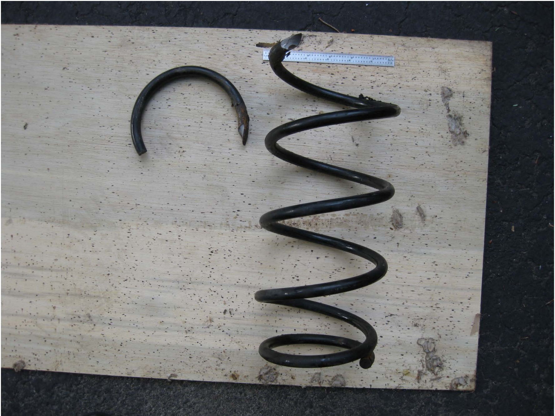
PASSENGER SIDE SPRING (right) – BROKEN PIECES
