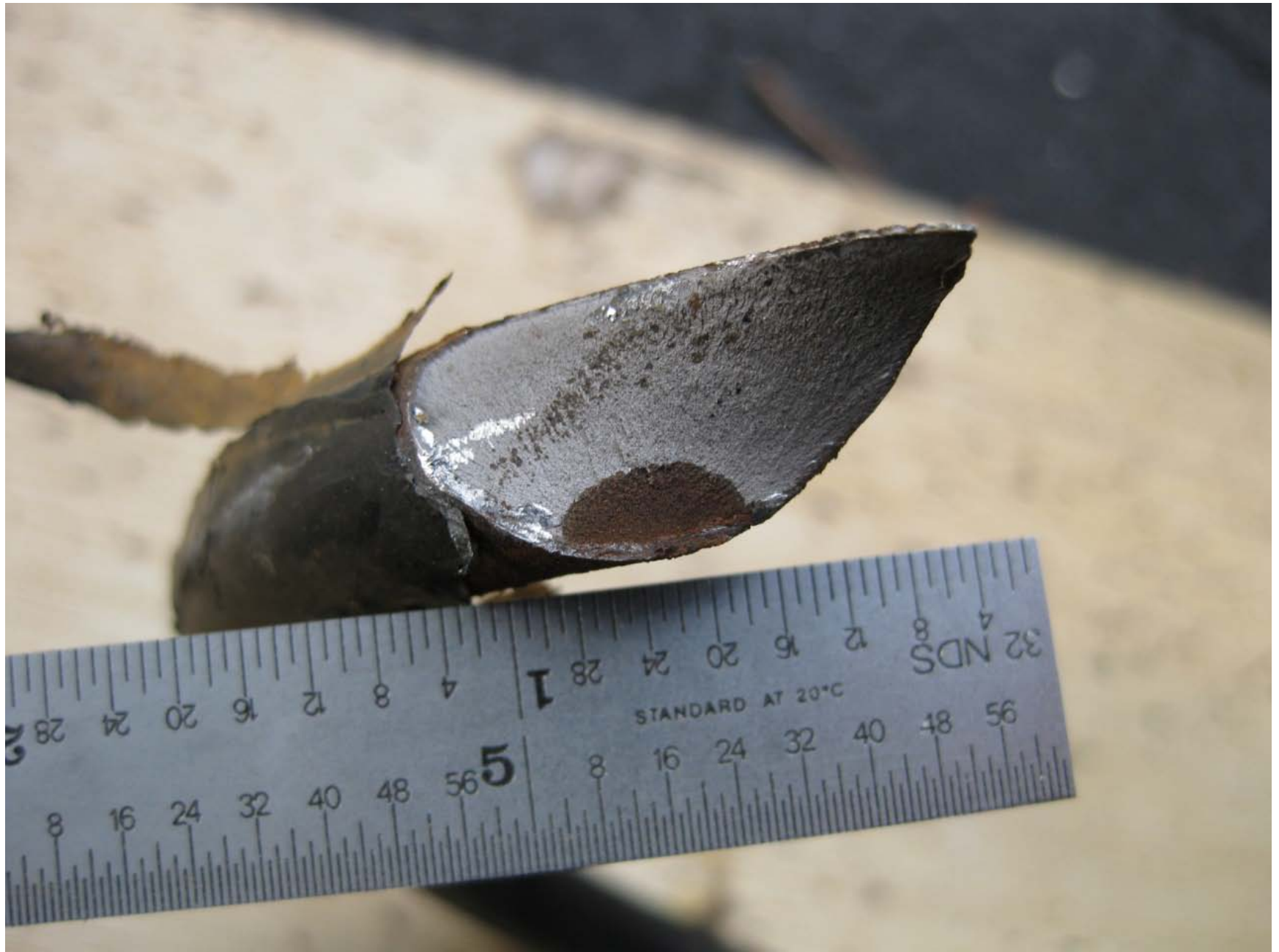
CLOSEUP OF BROKEN REGION OF LARGE SIDE OF BROKEN SPRING WITH SCALE
