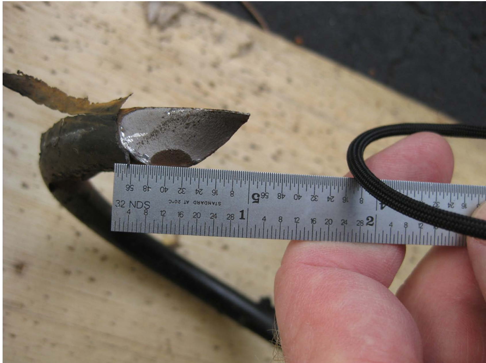
CLOSEUP II OF BROKEN COIL SPRING (FROM LARGE PIECE OF BROKEN SPRING)
