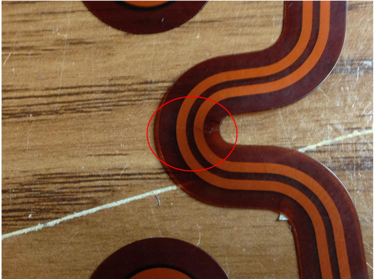
Attachment 2: Hairline Crack
