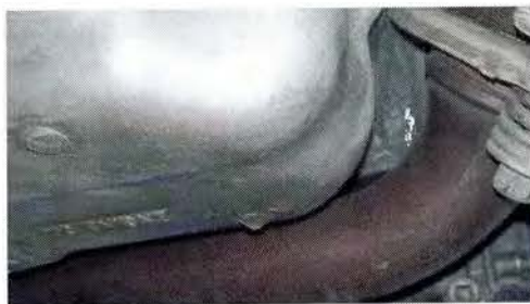
Oil pan and fluids dripping off of it
