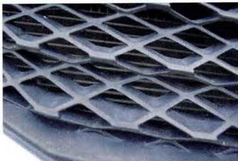
No signs of damage to grill
