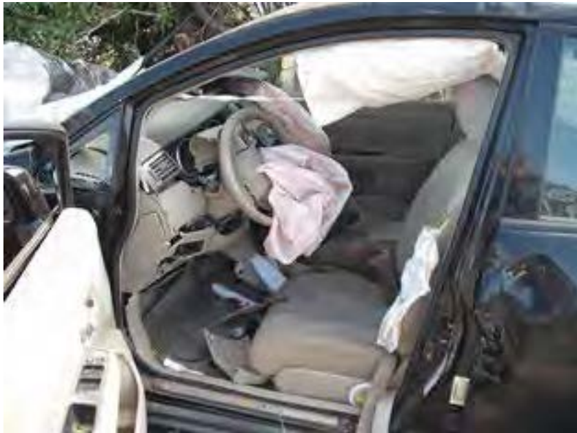
PHOTO OF UNIT 1 DEPICTING SIDE AIR BAG DEPLOYMENT & CUT SAFETY BELT
