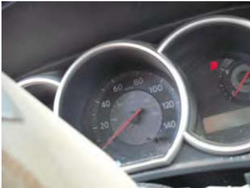
PHOTO OF UNIT 1'S INSTRUMENT PANEL DEPICTING NO POWER & LACK OF SPEED INDICATION
