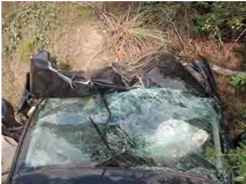
TOP VIEW OF UNIT DEPICTING DAMAGE TO UNIT 1'S FRONT END
