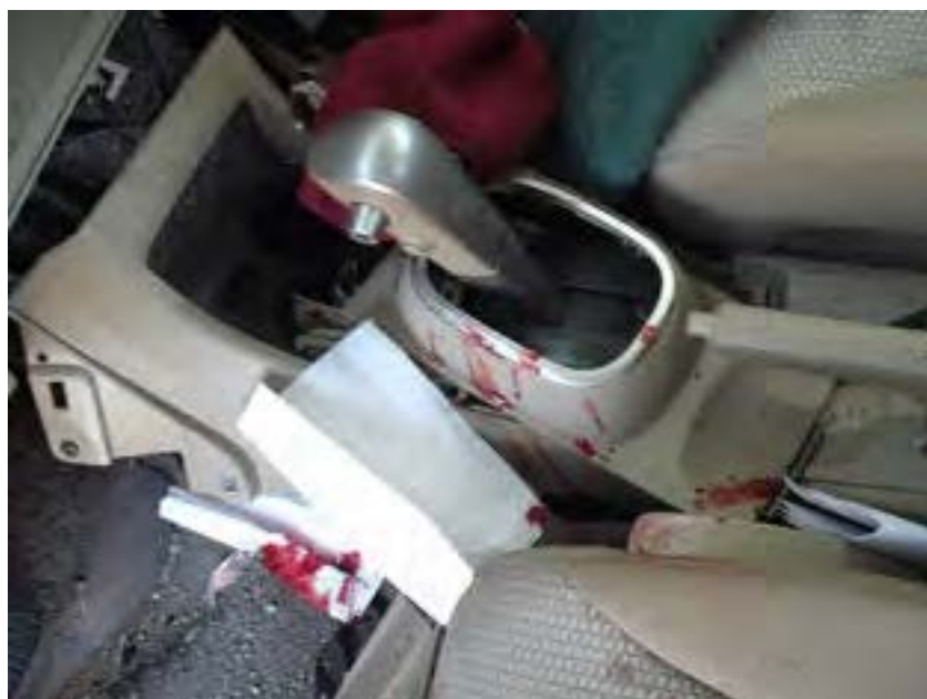
PHOTO OF UNIT 1'S CENTER CONSOLE INDICATING DAMAGE TO INTERIOR OF VEHICLE AND TRANSMISSION GEAR PLACEMENT
