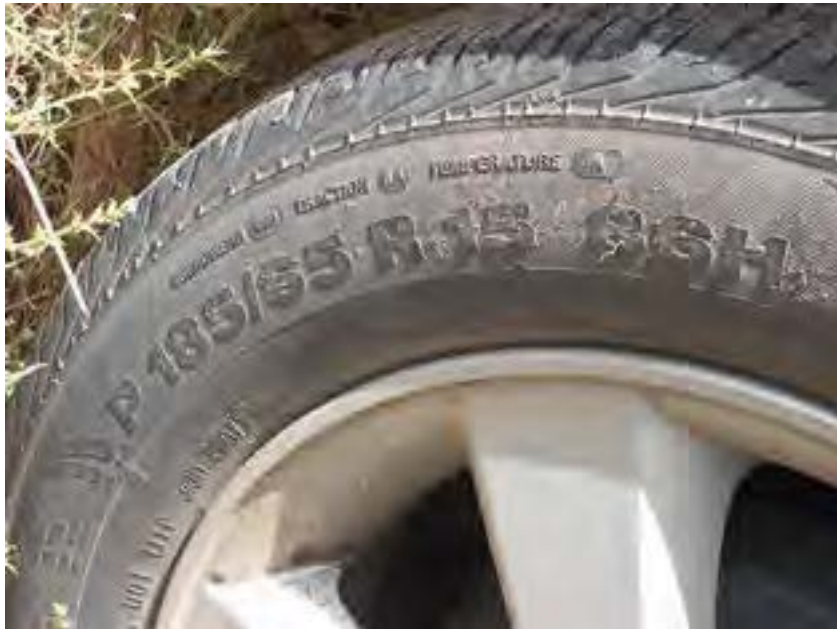
PHOTO OF UNIT 1'S RIGHT REAR TIRE DEPICTING THE VEHICLE'S TIRE SIZE
