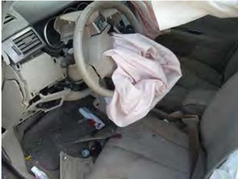
PHOTO OF UNIT 1 DEPICTING UNIT 1'S AIR BAG DEPLOYMENT & DRIVER SAFETY BELT
