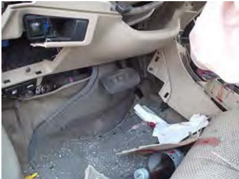
PHOTO OF UNIT 1'S DRIVER SIDE FLOOR BOARD DEPICTING PEDAL PLACEMENT POST CRASH & INTRUSION INTO THE VEHICLE
