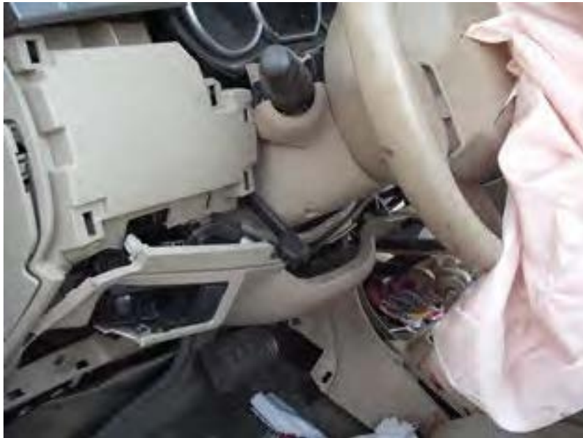
PHOTO OF UNIT 1'S DRIVER SIDE STEERING COLUMN DEPICTING DAMAGE TO VEHICLE CONTROLS & STEERING COLUMN
