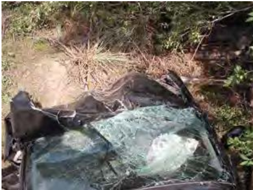
TOP VIEW OF UNIT 1'S FRONT END DEPICTING DAMAGE TO ITS RIGHT FRONT SIDE
