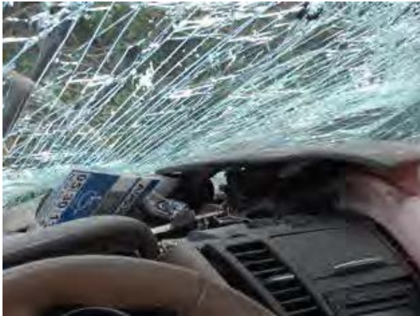
PHOTO OF UNIT 1'S WINDSHIELD DAMAGE & REAR VIEW MIRROR DISPLACEMENT
