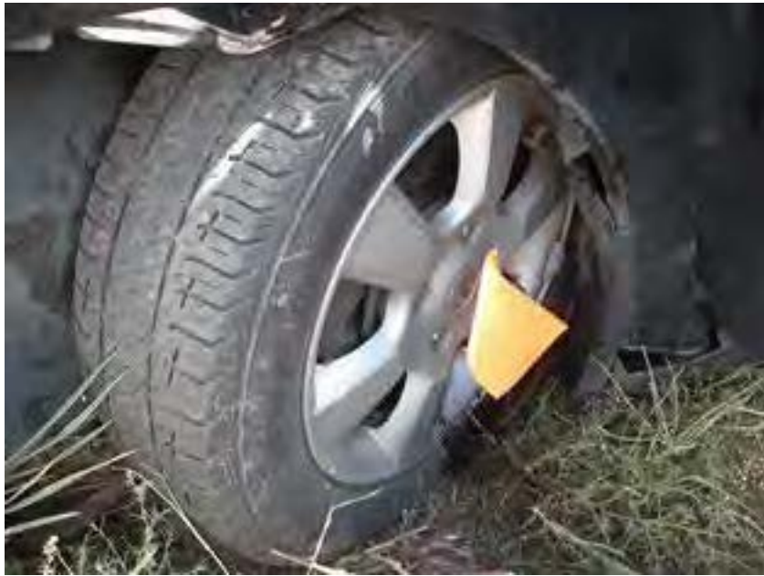
PHOTO OF UNIT 1'S LEFT FRONT TIRE AND WHEEL DEPICTING TYPE, SIZE, AND DAMAGE TO WHEEL WELL
