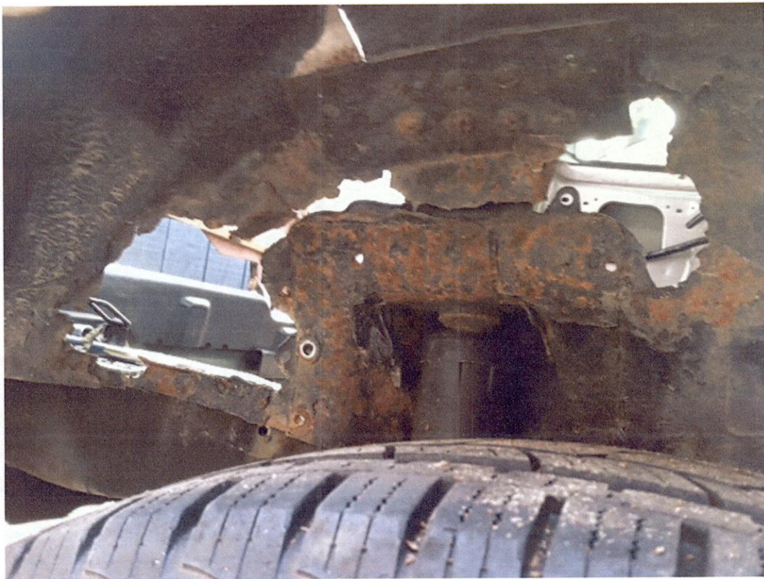
2004 Ford Escape: Rusted out shock mount and seat belt mount
