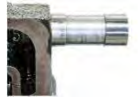
Valve body spool after transmission service
