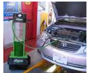
Coolant flush equipment
