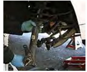
Worn out MacPherson struts
