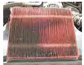
Dirty and restricted air filter
