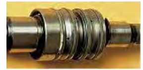
Power steering spool valve with hardened cracked seals
