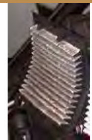
A dirty and clogged cabin air filter
