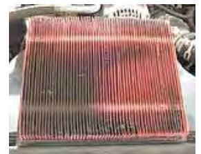
Dirty and restricted air filter
