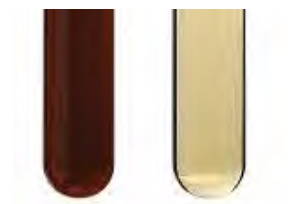
Brake fluid before and after service
