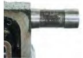
Valve body spool with heavy build up
