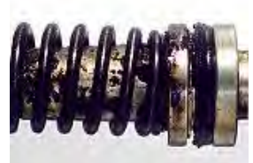
Harmful deposits on brake master cylinder piston assembly
