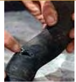
Worn out cooling hose
