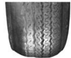
Abnormal tire wear from bad alignment
