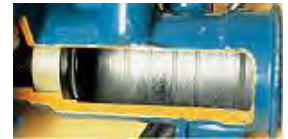
Grooves worn into the housing by hardened seals
