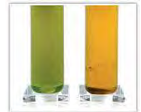
Clean vs. dirty, acidic coolant (antifreeze)
